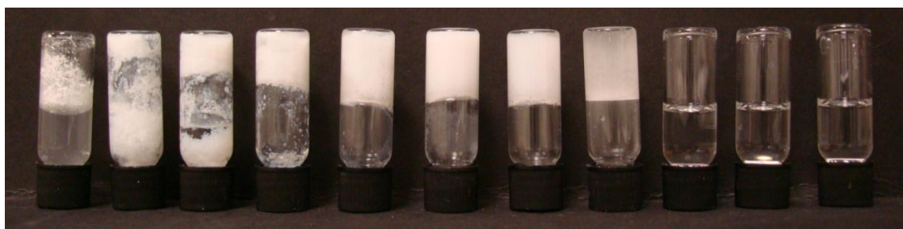
Figure S2. DMSO:Water gels formed by the addition of water to a solution of 1^2 in DMSO. From left to right the solvents are: pure water, ratios 1:9; 2:8; 3:7; 4:6; 5:5; 6:4; 7:3; 8:2; 9:1; pure DMSO. Note that the more aqueous samples, 1:9; 2:8; 3:7, are precipitated and/or form weak gels. Note the 8:2; 9:1 and pure DMSO samples are clear solutions.
