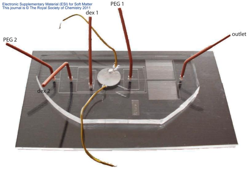
PDMS-on-glass chip used for the forced formation of core-shell double emulsions all aqueous microdrops. Solutions of PEG and dextran are fed into the four orange tubes on the left. Forced formation occurs by the contraction of a piezo electric bending disc embedded in the PDMS, which is actuated by applying a sinusoidal voltage to it through the two yellow wires. After their formation, drops flow through a channel with a length of 80 cm before leaving the device through the exit tube.
