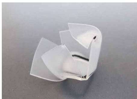
Figure S3. Photograph of a deformed box that is representative of the deformation that occurs to the panels when a sample is over-exposed to the light from the IR lamp.
