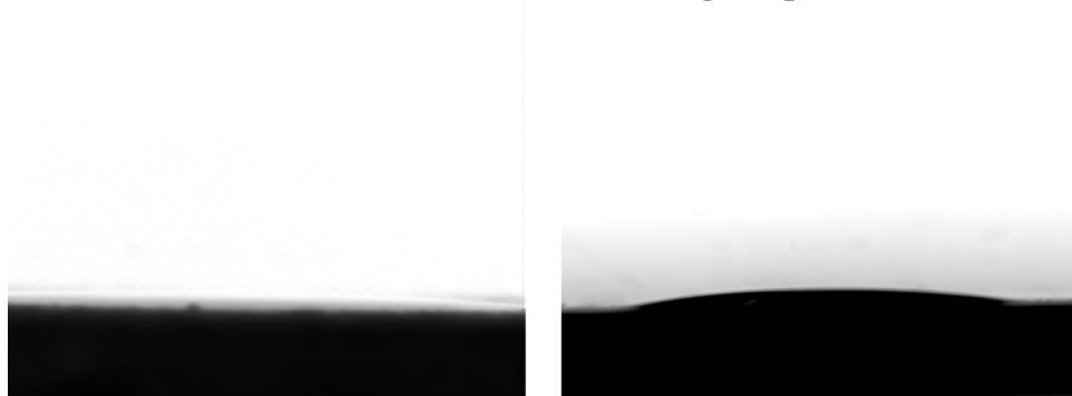
**Fig. S2** Oil droplets on (a) a polystyrene/nanoparticle composite coated plate and (b) a flat glass plate in atmosphere. The composite coatings and glass plates both showed oleophilic properties.
