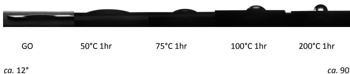
Fig. S5 Pictures shows the increasing contact angles of a GO thin film with respect to increasing heating temperature.
