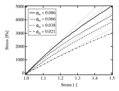
The stress-strain curve of Tetra-PEG gel 20k ( $\phi_0 = 0.034$ ), with different  $\phi_m$ 's. The thin dotted lines show the fit results.
