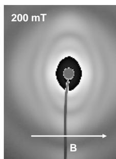
Figure S2: Detector image of a SAXS measurement of silica-coated maghemite ellipsoids suspended in water with an applied magnetic field of 200 mT pointing in the indicated direction.
