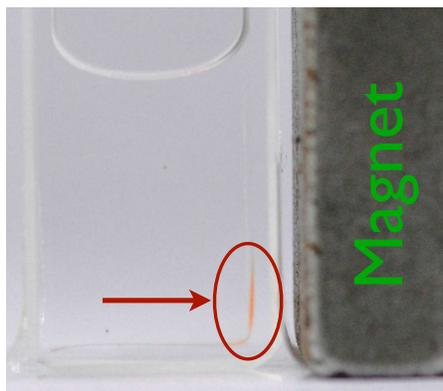
Figure S3: SCM-PNIPAM colloids in aqueous suspension isolated on the wall of the glass vial next to a permanent magnet.
