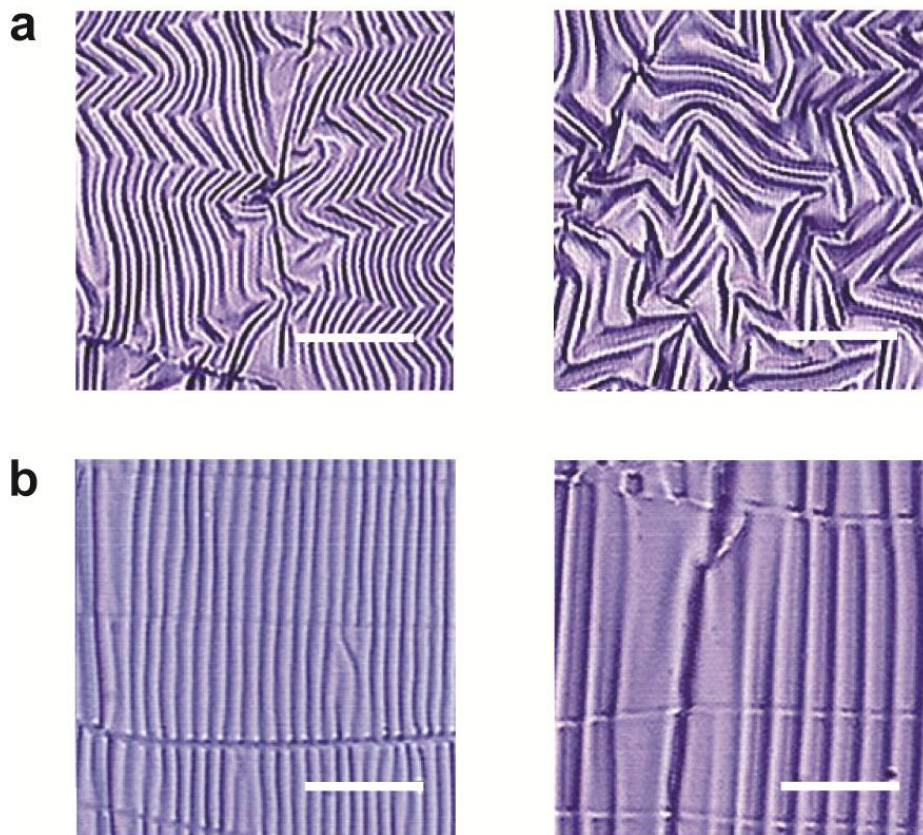
Figure S5. Optical images for wrinkle patterns with bending strains. a. Convex bending strain. b. Concave bending strain. Left images of a, b: bending angle 45^\circ . Right image of a, b: bending angle: 60^\circ . Flame exposure time: 30 s. All scale bars: 20\ \mu\text{m} .
