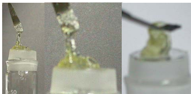
Fig. S6 Pictures of the 1 gel in toluene, indicating the good gel state of 1 when a small strain was imposed.
