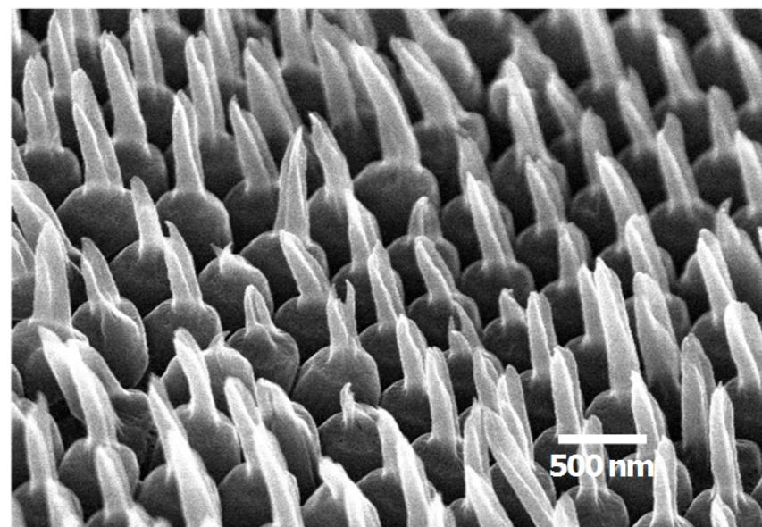
**Figure S1.** SEM image of PS nanohairs peeled off from an untreated multi-branched AAO template with multi-branching.
