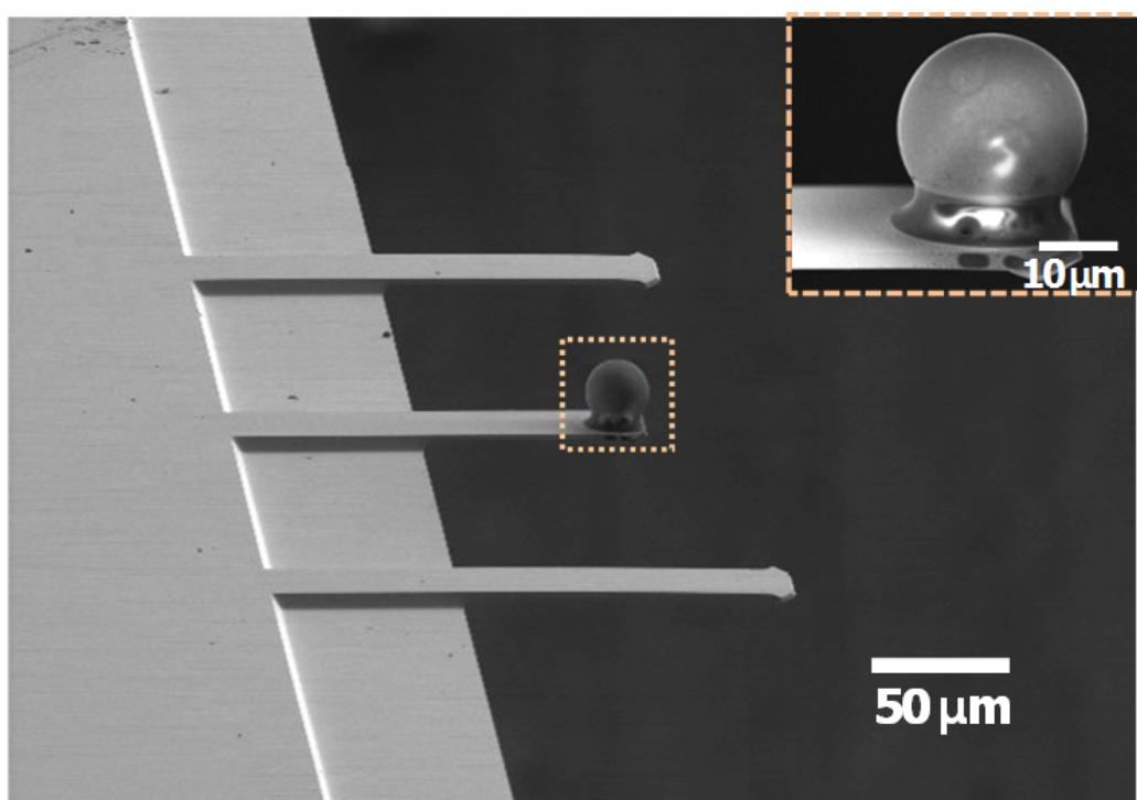
**Figure S2.** SEM image of the cantilever tip modified with a silica ball (24  $\mu\text{m}$  in diameter).
