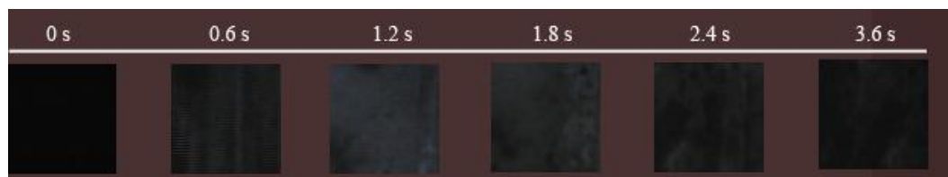
Fig. S4. Photos showing the transparency change in the deswelling process of grafted PNIPAAm at 50 °C. The sample used was photografted in 2 mol/L NIPAAm solution for 10 min.
