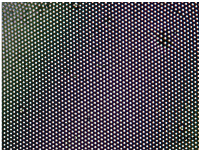
Silk fibroin film with convex microlens patterning obtained by casting from water solution on a PS template pre-treated with MeOH
