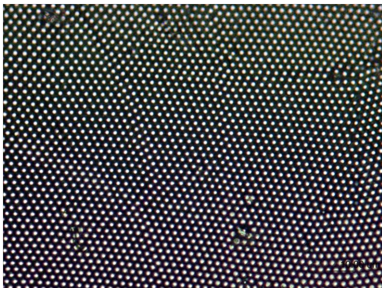
Silk fibroin film with convex microlens patterning obtained by casting from water solution on a PS template pre-treated with plasma
