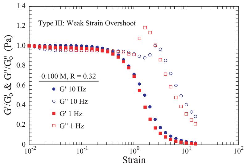
Figure 2: Reduced moduli  $G'/G'_0$  and  $G''/G''_0$  vs strain amplitude for the 0.100 M CTAB,  $R = 0.32$  solution at high oscillation frequencies: 1 Hz, and 10 Hz.
