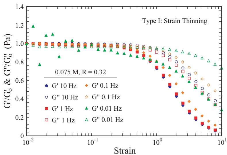
Figure 3: Reduced moduli  $G'/G'_0$  and  $G''/G''_0$  vs strain amplitude 0.075 M CTAB,  $R = 0.32$  solution at different oscillation frequencies: 0.01 Hz, 0.1 Hz, 1 Hz, and 10 Hz.
