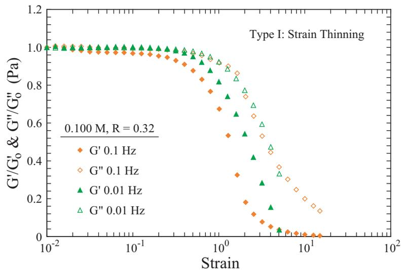
Figure 1: Reduced moduli  $G'/G'_0$  and  $G''/G''_0$  vs strain amplitude for the 0.100 M CTAB,  $R = 0.32$  solution at low oscillation frequencies: 0.01 Hz, 0.1 Hz.
