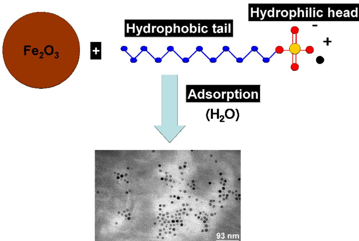
**Figure S1.** Scheme of the different steps of the preparation of the suspension and TEM image of SDS modified maghemite nanoparticles (SDS-NPs).
