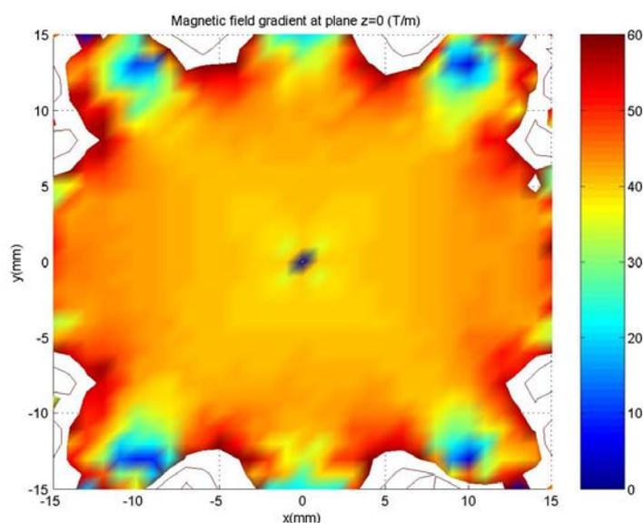
**Figure S4.** Distribution of the radial gradient magnetic field in the SEPMAG LAB 1x25 ml 2042 plus system (60T/m)
