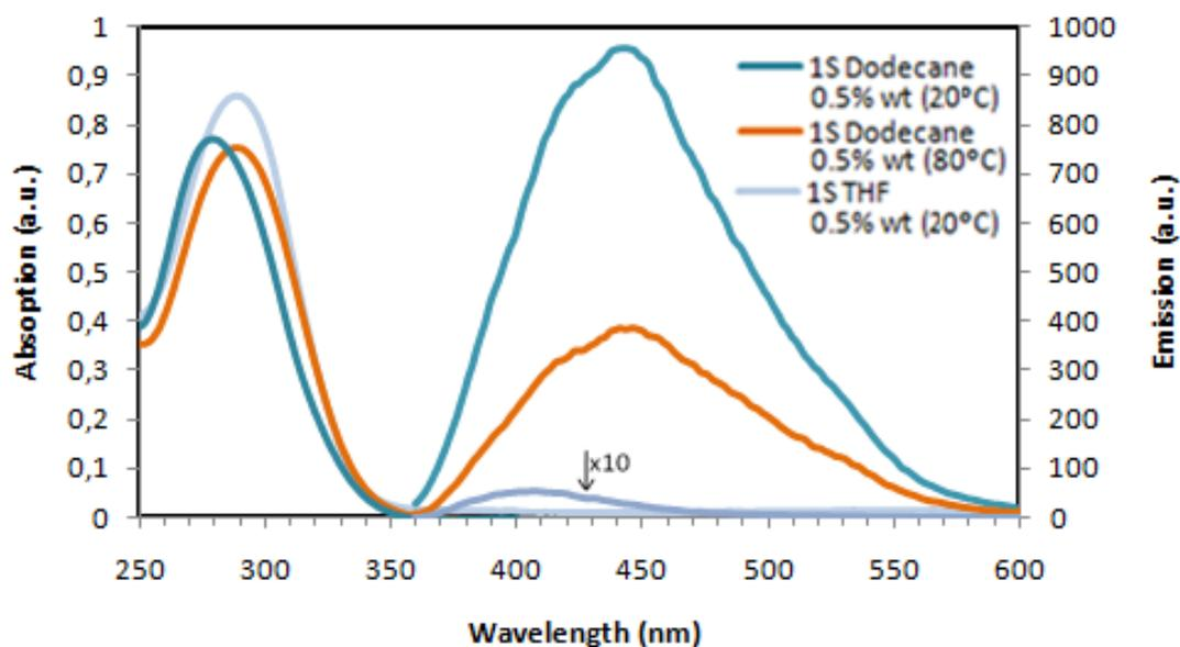
**1R** in the gel state (dodecane, 0.5 % wt). Fluorescence change with temperature on heating.
