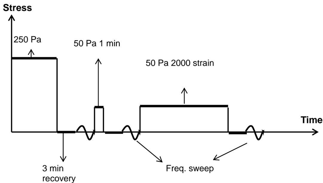
**Figure S1:** Shear history imposed upon the samples. The small amplitude oscillatory tests were done with 10% strain and in the frequency range of 100 to 0.1 rad/sec. Only the last frequency sweep test is discussed in this paper. The morphology was measured on samples quenched after the last frequency sweep test.
