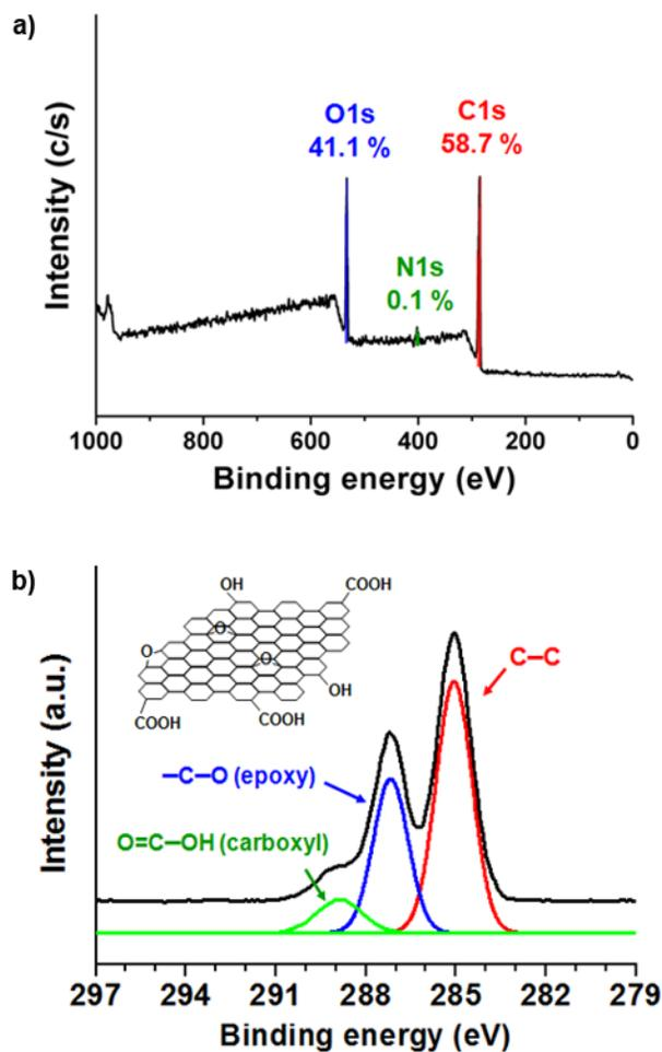
**Fig. S1.** a) XPS Survey of GO sheets oxidized graphene discs and b) XPS C1s spectra of GO sheets.
