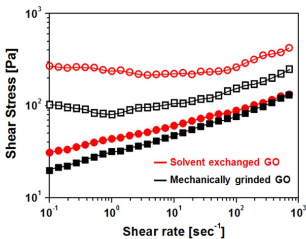
**Fig. S2.** Shear stress for the 5 wt% of GO sheet-based ER fluids under electric field strength (5 kV/mm). Open and closed symbols indicate with and without electric field strengths, respectively.
