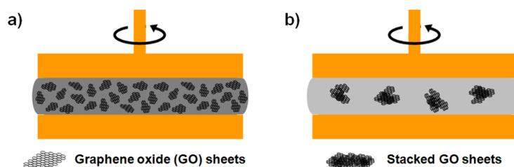
**Fig. S3** Schematic illustration for the dispersing state of (a) solvent exchanged GO sheets and (b) mechanically grinded GO sheets.
