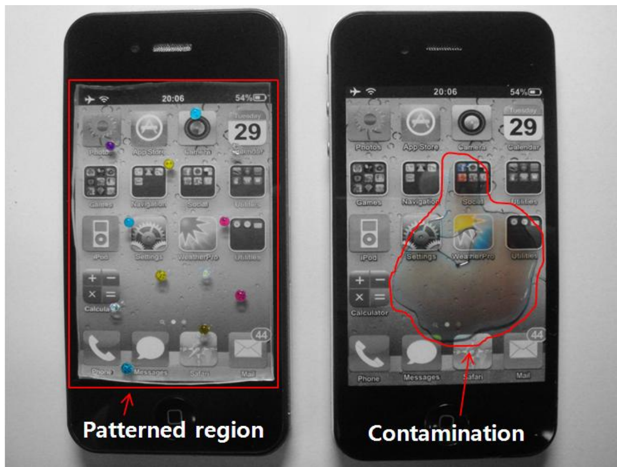
Figure S4. Demonstration of superomniphobic surfaces on touch-phone screens. The left figure shows that the superoleophobic surface (PDMS micropillar arrays, SR = 6 ) is not contaminated by various liquids: DI water (transparent), mineral oil (blue), hexadecane (red) and ethanol (yellow). In contrast, the unmodified surface on the right is immediately wetted by the liquids upon contact.
