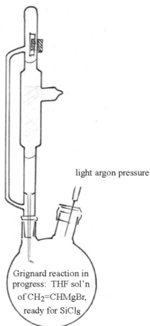
**Figure S4.** Chlorosilane transfer technique, scene 3.
