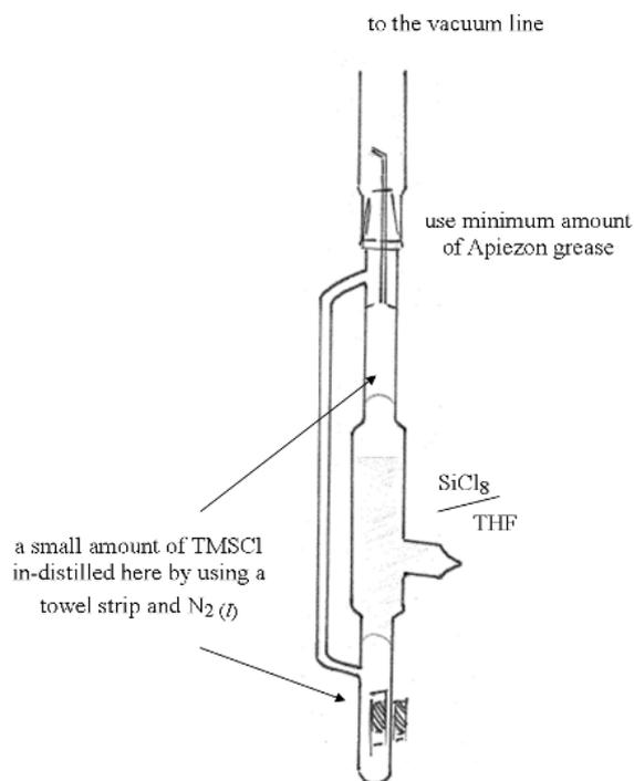
**Figure S3.** Chlorosilane transfer technique, scene 2.
