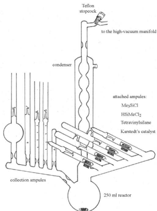
**Figure S1.** Hydrosilylation apparatus.
