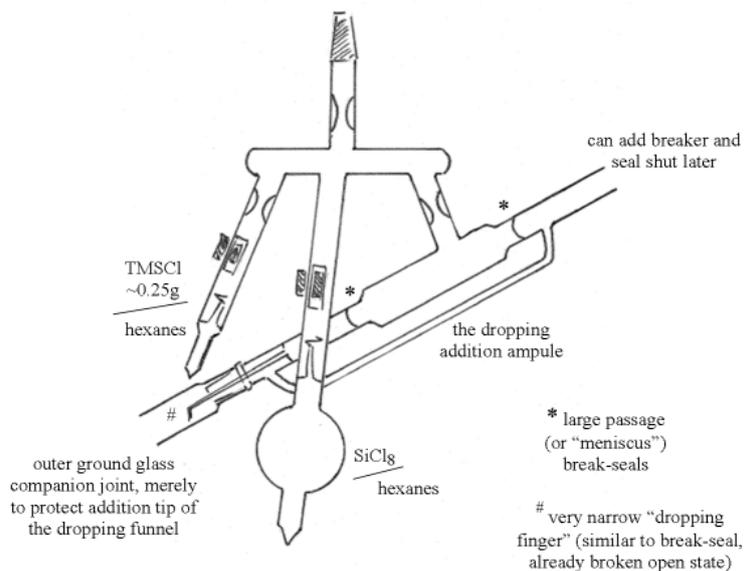
**Figure S2.** Chlorosilane transfer technique, scene 1.
