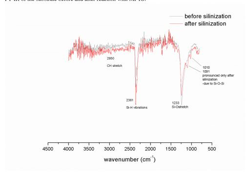
Successful chemical modification of the surface with MPTS can be determined by the appearance of peaks (red trace) after silinization at 1010 and 1091 cm<sup>-1</sup> which correspond to Si-O-Si bonds. The small CH stretch from MPTS can be observed at 2950 cm<sup>-1</sup>.
