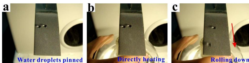
Supplementary Figure S1. Digital images of in-situ hot effects induced reversible adhesion by directly heating.
