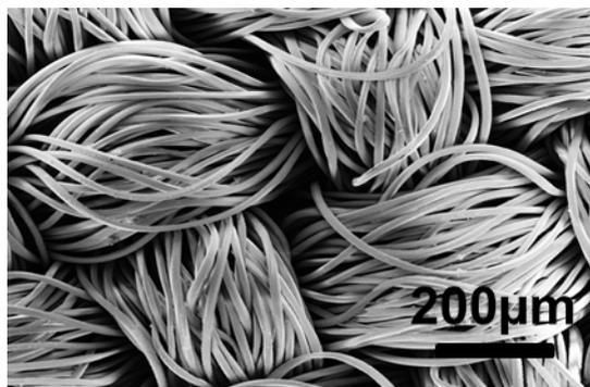
Fig. S1 SEM image of uncoated polyester fibres.
