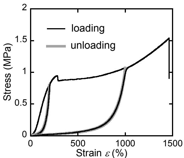
**Figure S1** Tensile loading-unloading curves of the DN gel. Strain was calculated from the cross-head displacement, different from the other experiments in main text. The loading and unloading curves were overlapped each other even in large strain. Tensile velocity was fixed at 100 mm/min.
