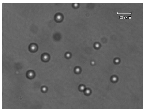
**Figure S3.** Light microscope photos of microcapsules prepared with PDADMAC-TC4.
