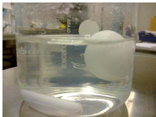
**Figure S1.** Result of microencapsulation using PDADMAC in the water phase.
