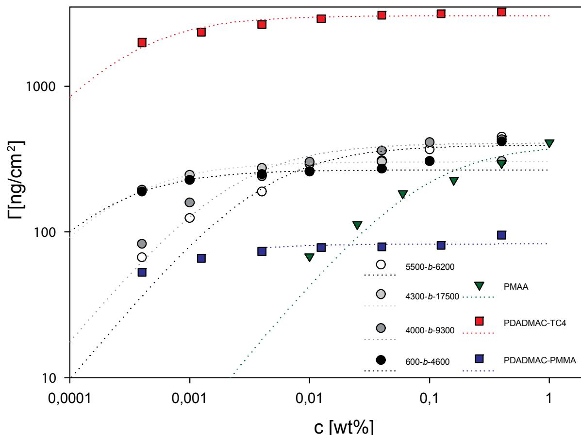
**Figure S5.** Adsorption isotherms on a log-log scale of 600-*b*-4600 (●), 4000-*b*-9300 (●, dark grey), 4300-*b*-17500 (●, grey) 5500-6200 (○, white), PMAA (▼, green), PDADMAC on a TC4 modified PMMA surface (■, red) and PDADMAC on a pure PMMA surface (■, blue) as measured with QCM-D.
