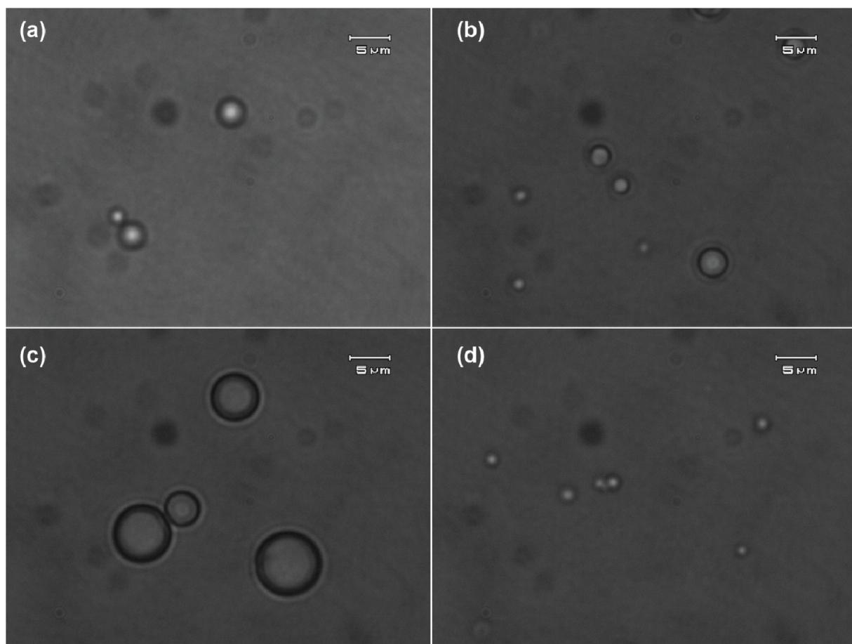
**Figure S2.** Light microscope photos of microcapsules prepared with different dispersants; a) PMAA, b) 600)-*b*-4600, c). 4000-*b*-9300 and d) 4300-*b*-17500.
