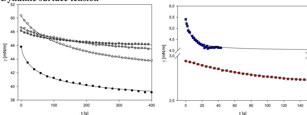
**Figure S4.** Oil-water interfacial tension decay for the different dispersant systems. Left; 600-b-4600 (●), 4000-b-9300 (○, dark grey), 4300-b-17500 (●, grey) 5500-6200 (○, white). Right; w(PDADMAC)-o(TC4) (■, red) and w-o(TC4) (■, blue).
