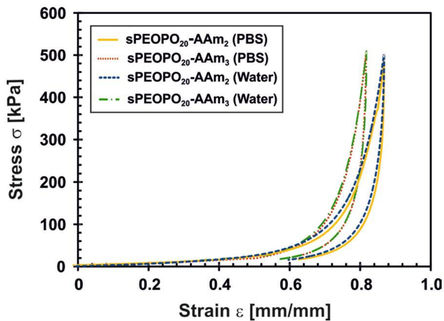
**Figure S2:** Hysteresis cycles of sPEOPO<sub>20</sub>/AAm<sub>Y</sub> DN hydrogels (Y = 2 and 3 M AAm) accomplished under distilled water and PBS surroundings.
