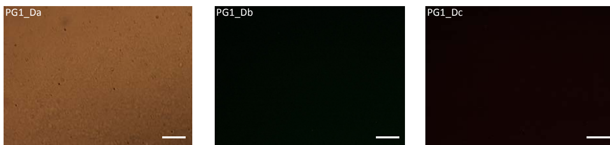
Figure S4. Microscope images for control of PG1 treated with D (100 % FAM- \text{DNA}_S ) after 3 washes with incubation buffer. 100x magnification, scale bar 100 \mu\text{m} . As expected no fluorescence was observed. PG1_Da : White light microscopy image for PG1 (D, treated with 100 % FAM-DNA), PG1_Db : Fluorescence
