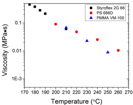
**Figure S3.** Melt flow index for Styroflex 2G 66 and confining layer PS and PMMA. Processing temperatures: ~ 210 °C for STF and PMMA and 220 °C for PS.
