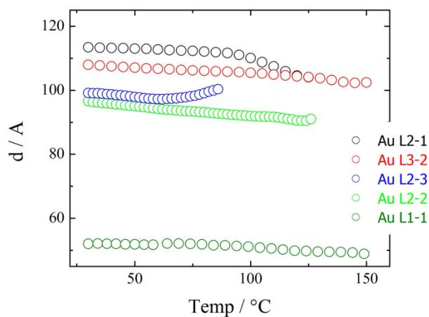
**Figure 1.** Layer spacing dependence on temperature for lamellar phases of studied hybrid materials.
