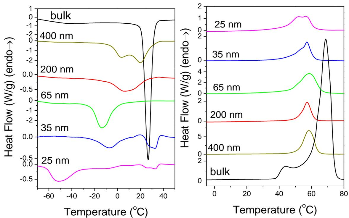
**Fig. S2.** Cooling (left) and subsequent heating (right) thermograms of bulk PCL-36000 and PCL-36000 located inside self-ordered AAO with pore diameters ranging from 200 nm to 25 nm. (heating/cooling rate 10 K/min).`
