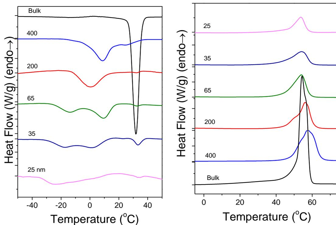
**Fig. S3.** Cooling (left) and subsequent heating (right) thermograms of bulk PCL-7700 and PCL-7700 located inside surface-modified with ODPA self-ordered AAO with pore diameters ranging from 400 nm to 25 nm (heating/cooling rate 10 K/min).
