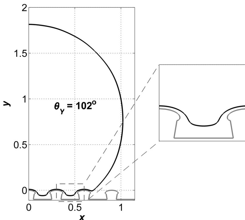
**Fig. SI 4** Equilibrium solution of a cylindrical droplet wetting a mushroom-like striped surface. The material wettability corresponds to  $\theta_Y = 102^\circ$ . The inset shows a magnified view of the cross-section of each mushroom-shaped stripe.
