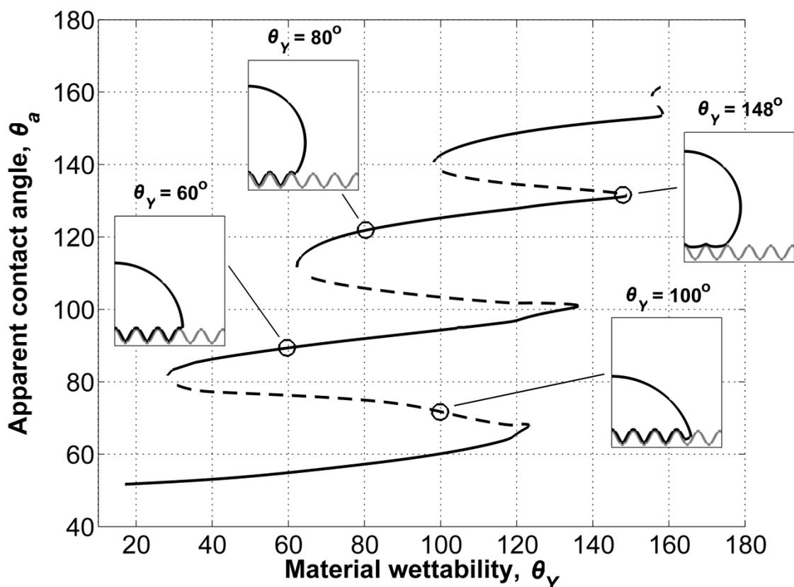
Fig. SI 3 Dependence of the droplet height on the material wettability ( $\theta_Y$ ) for a concentric rings-patterned solid surface (eq. (17) with  $p_4 = 8$ ,  $p_5 = 2$ ).
