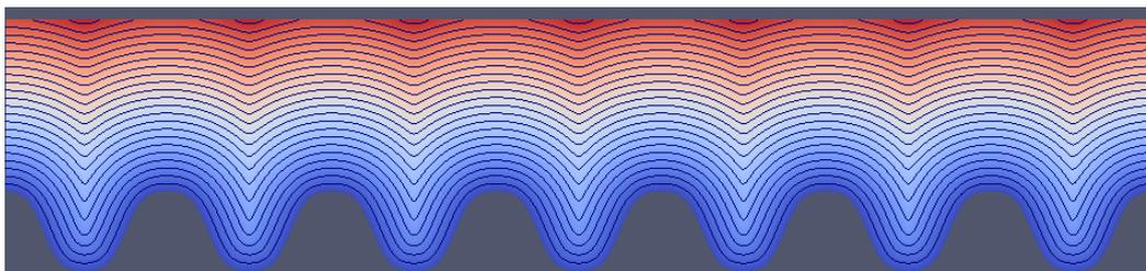
**Fig. SI 5** Contour lines of constant distance,  $\delta$ , from the solid boundary obtained from the Eikonal equation solution. The topography of the solid surface is given by eq. (18).
