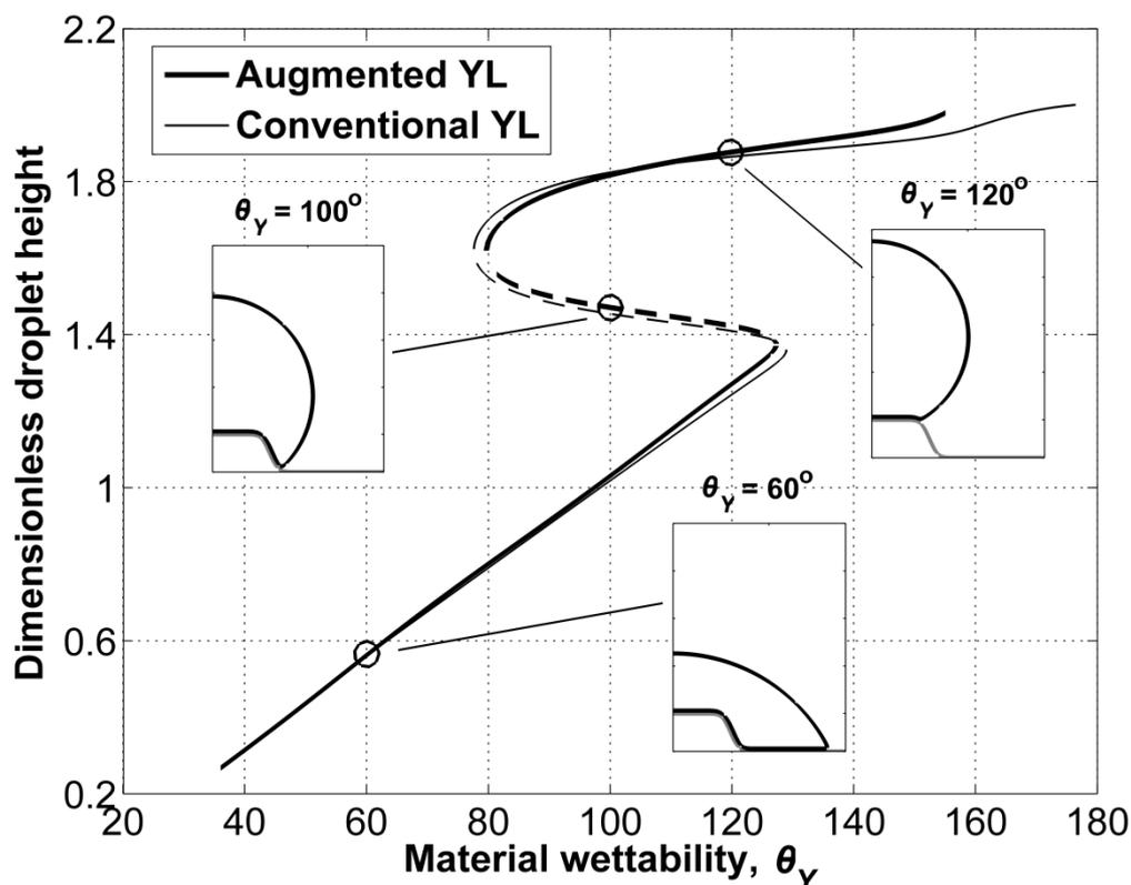
**Fig. SI 2** Dependence of the droplet height on the material wettability ( $\theta_Y$ ) for a single-pillared solid surface structure (eq. (16) with  $p_1 = 0.6$ ,  $p_2 = 10$ ,  $p_3 = 5$ ).
