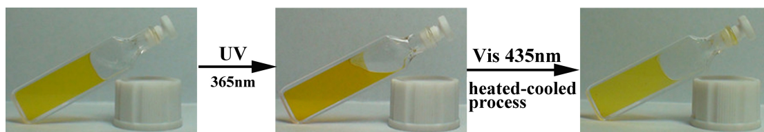
Fig. S4 Pictures of the gel-sol-gel transitions of the ethyl acetate gel of CAZODA, showing the reversibility of the gel.
