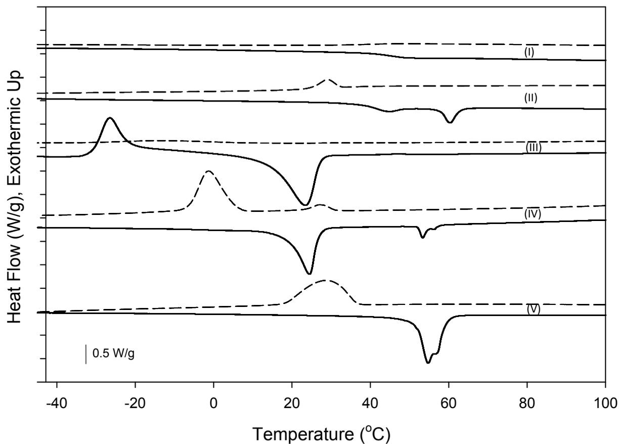
**Figure S5.** DSC thermograms of 1<sup>st</sup> cooling (dashed line) and 2<sup>nd</sup> heating (solid line) for: (I) PPG-EP, (II) PPG-EP/10%-PCL, (III) PEO/EP, (IV) PEO-EP/10%-PCL, and (V) PCL. Heating rate of 10 °C/min was used for cooling and heating of both samples. It is noted that the heat flow magnitude of the DSC thermogram for PCL was reduced by half for scaling purposes.
