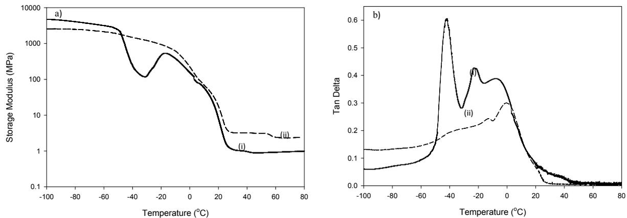
**Figure S6.** (a) Tensile storage modulus ( $E'$ ) and (b) loss tangent ( $\tan \delta$ ) trace of PEO-EP/PCL with different PCL content in comparison with neat epoxy PEO-EP, measured by DMA. (i) PEO-EP and (ii) PEO-EP/10%PCL.
