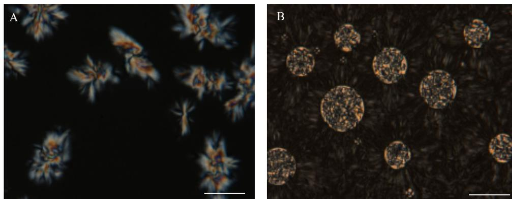
**Figure S1.** POM images under crossed polarizers exhibited by: (A) PPG-EP/PCL and (B) PEO-EP/PCL. The scale bar represents 50  $\mu\text{m}$ .
