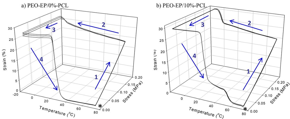
**Figure S7.** The triple-shape memory cycle of PEO-EP/PCL with (a) 0% and (b) 10% PCL content using one-step fixing. The beginning of the cycles are marked by the asterisk. Samples were loaded to a tensile strain of 20%, cooled to  $-10$  °C and unloaded (fixing), followed by continuous heating to  $75$  °C (recovery). The arrows denote the various stages, specifically (1) deformation, (2) fixing, (3) unloading, and (4) recovery.
