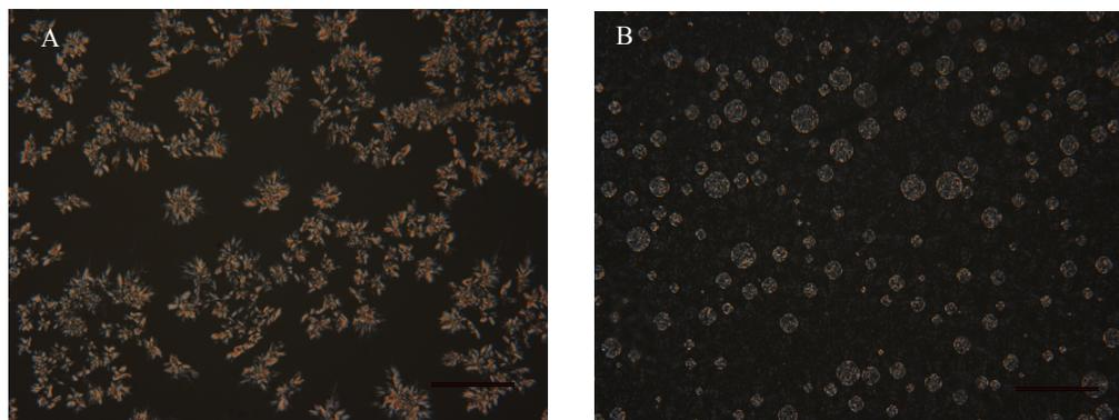
**Figure S2.** POM images under crossed polarizers exhibited by: (A) PPG-EP/PCL and (B) PEO-EP/PCL. The scale bar represents 200  $\mu\text{m}$ .
