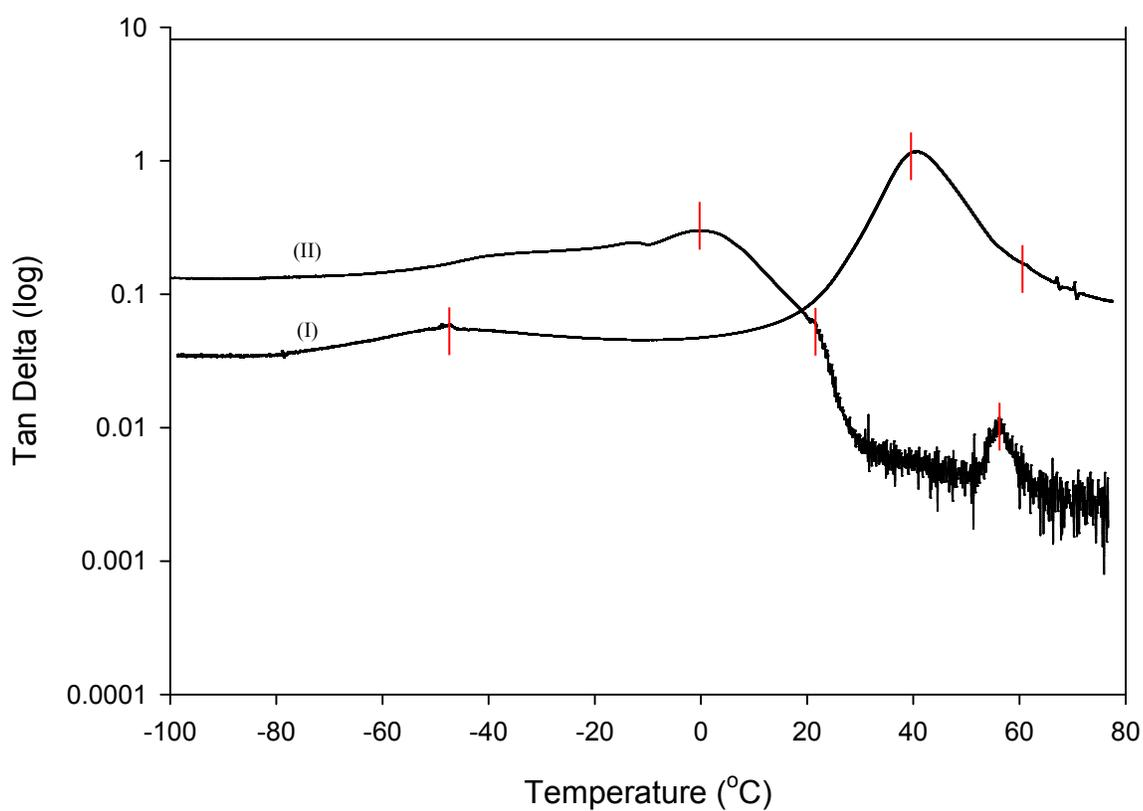
**Figure S4.** DMA loss tangent ( $\tan \delta$ ) trace of (I) PPG-EP/PCL and (II) PEO-EP/PCL in log scale demonstrating all three transition temperatures. Red lines show the transition temperatures of each composite.
