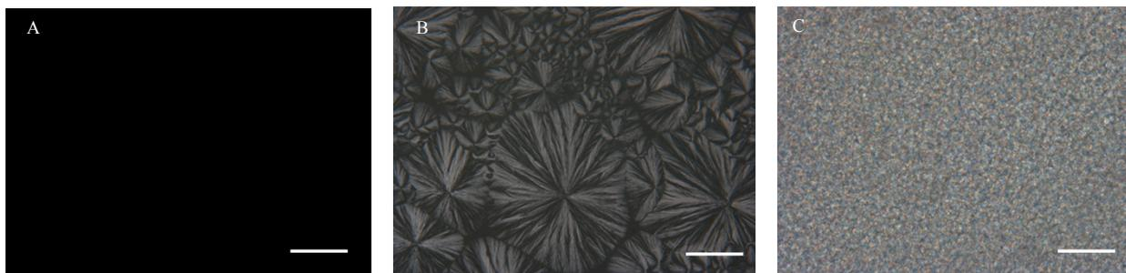
**Figure S3.** POM images under crossed polarizers at room temperature exhibited by: (A) PPG-EP, (B) PEO-EP, and (C) PCL. The scale bar represents 200  $\mu\text{m}$ .
