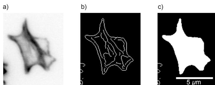
Figure S2: Pictures of different steps in image processing. a) Original TxRed-image of actin structures of the cell, inverted. b) Detected outlines by canny algorithm (in MATLAB). c) Binarized image (in ImageJ) after manually closing outlines detected by the canny algorithm.
