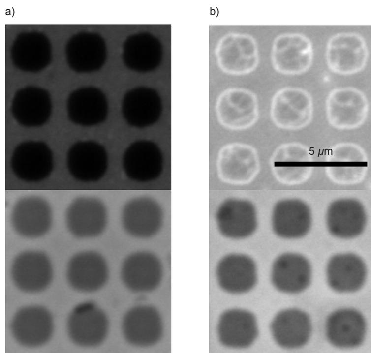
Figure S1: Micrographs showing the coating quality. The substrates have been coated as described in section Substrate Preparation. a) Fluorescence and phase contrast images of a microcontact-printed (structured, selectively-coated) substrate. b) Fluorescence and phase contrast images of a fibrinogen-coated (structured, completely coated) substrate.
