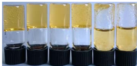
Figure S7. Gel-sol phase transition of gel 2 (3.01 mM in isopropanol/water = 1:1) triggered by different equivalent of \beta -CD (from left to right, in order, were 0 eq, 1 eq, 2 eq, 3 eq, 4 eq, 5eq).
