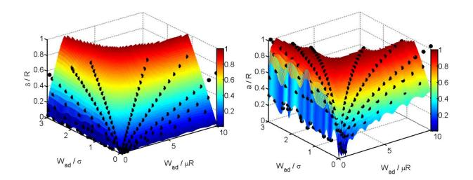
FIG. 7. The surfaces of indentation depth (left) and contact radius (right) are interpolated over a grid of  $(W_{ad} / \mu R, W_{ad} / \sigma)$ . The color maps indicate values of  $\delta / R$  and a / R. The scattered black dots are results from FEM simulations.
