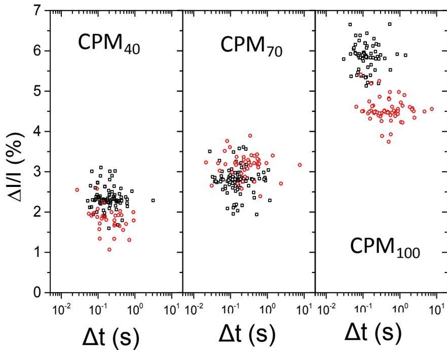
Fig. SI-5 : Relative current blockade vs dwell time induced by CMP translocation through native (black square) and TMS nanopores (red round)
