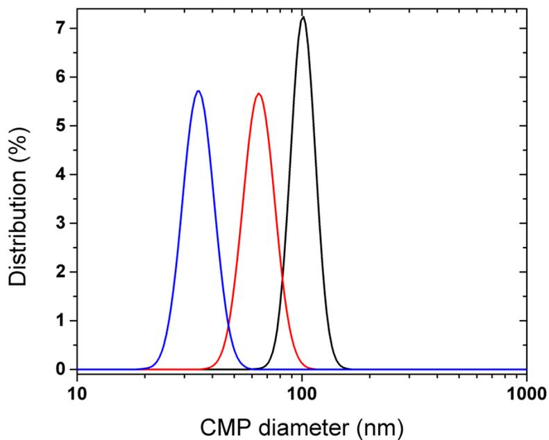
Fig. SI-2: Diameter distribution of the CMP obtained by PCCS (CMP<sub>40</sub> line blue, CMP<sub>70</sub> line red and CMP<sub>100</sub> line black)
