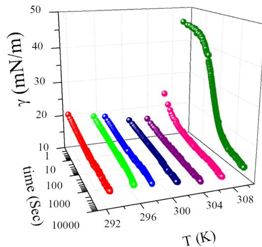
**Fig. S7** Three dimensional plots of the heptane-water  $\gamma_t$ -time-temperature in the presence of PNIPAM microgel dispersed in 0.5 mM NaCl solution (Note the minimum was observed at 304 K).
