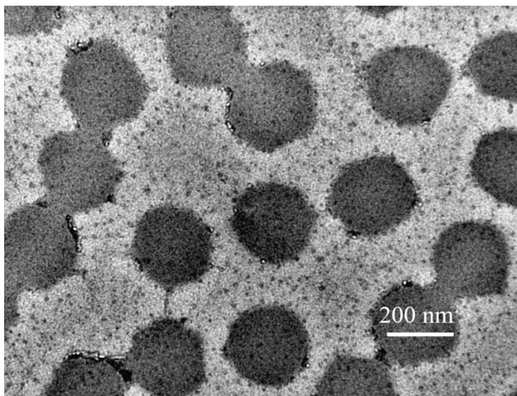
**Fig. S2** The typical image of the 3.2%BA microgels measured by TEM.
