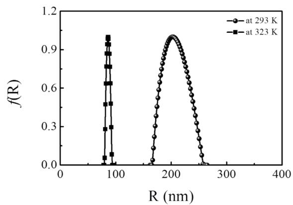
**Fig. S1** The typical hydrodynamic radius distribution of 3.2%BA microgels at 293 and 323 K, respectively, as measured by dynamic laser light scattering.
