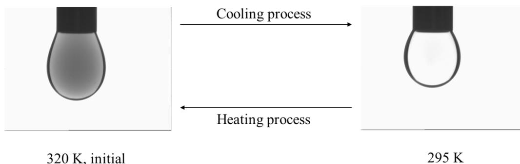
**Fig. S13** Single droplet experiment starting from 320 K: the droplet was cooled to 295 K and then heated back to 320 K.
