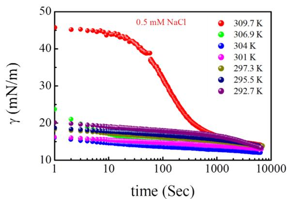
**Fig. S6** Temperature dependence of  $\gamma_t$  in the presence of PNIPAM microgel dispersed in 0.5 mM NaCl solution.
