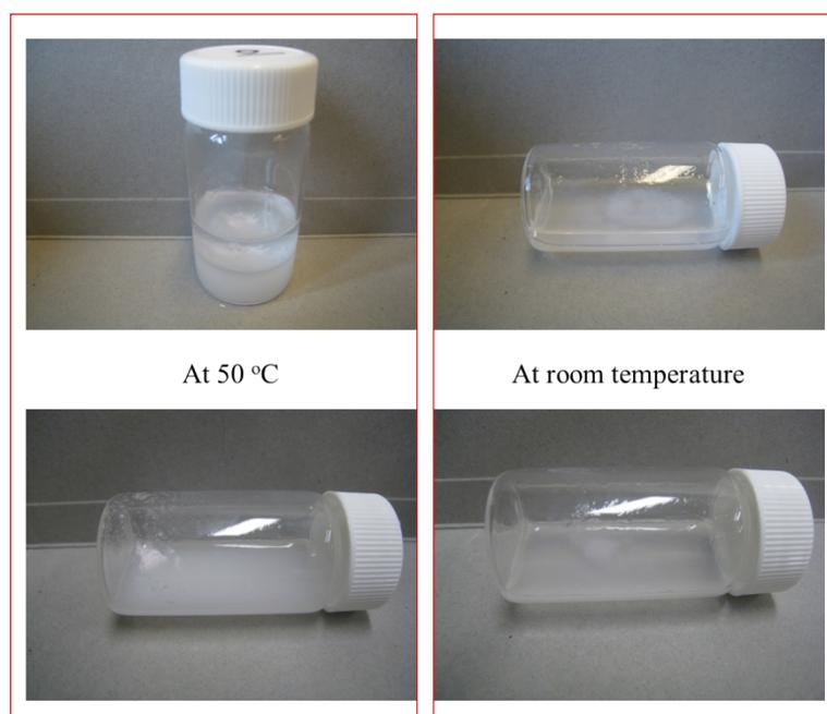
**Fig. S11** The appearances of 3.2%BA microgel aggregates at the heptane-water interface and at the water-air interface with microgels dispersed in 10 mM NaCl at 50 °C (right box). Note that these aggregates were still observable after the temperature cooled to room temperature and stayed for 24 hours (left box).
