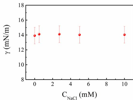
**Fig. S5** The effect of NaCl on  $\gamma_m$  in the presence of  $5 \times 10^{-3} \text{ g/mL}$  PNIPAM microgels at 298 K.
