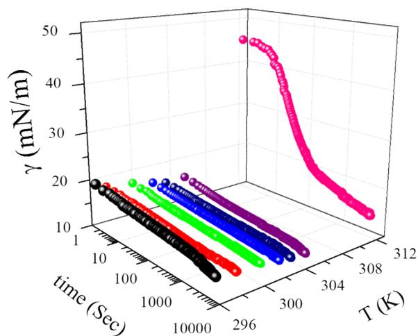
**Fig. S8** Three dimensional plots of the heptane-water  $\gamma_t$ -time-temperature in the presence of PNIPAM microgel dispersed in 2.75 mM NaCl solution (Note the minimum was observed at 305 K).
