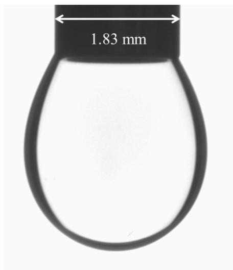
**Fig. S3** The typical pendant droplet used for the investigation of PNIPAM microgel behaviors at the heptane-water interface, at 294 K.
