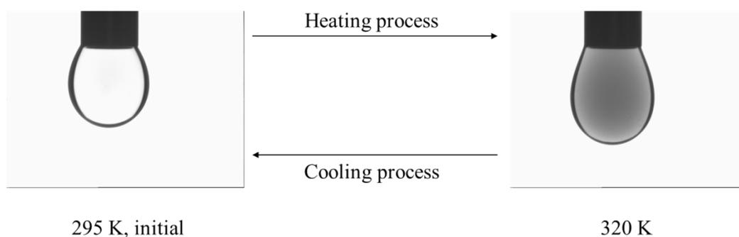
**Fig. S12** Single droplet experiment starting from 295 K: the droplet was heated to 320 K and then cooled back to 295 K.
