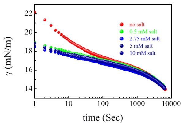
**Fig. S4** The NaCl salt concentration dependence of the heptane-water dynamic interfacial tensions ( $\gamma_t$ ) in the presence of PNIPAM microgels at 298 K.
