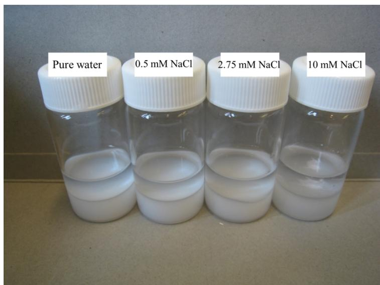
**Fig. S10** The appearances of heptane-water interface of 3.2%BA PNIPAM microgels dispersed at various NaCl solutions. Note that aggregates were only found when microgels were dispersed in 10 mM NaCl solution after heating the temperature above VPTT (50 °C).
