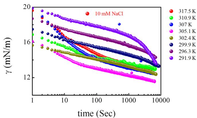
**Fig. S9** Temperature dependence of  $\gamma_t$  in the presence of PNIPAM microgels dispersed in 10 mM NaCl solution.
