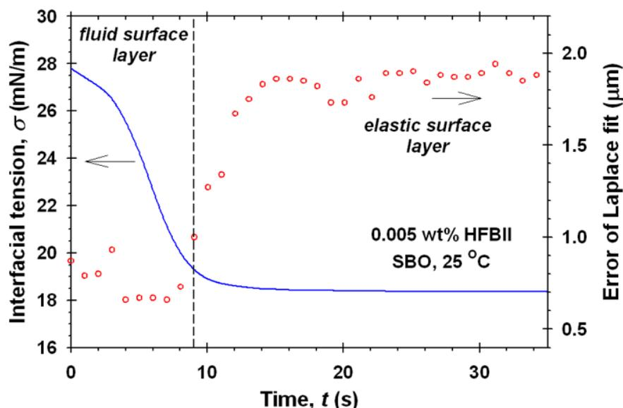
**Fig. B1.** Time dependencies of the interfacial tension and of the error of the fit of the drop profile by means of the Laplace equation: pendant drop method + DSA at 0.005 wt% HFBII in the water phase; the oil phase is soybean oil (SBO).
