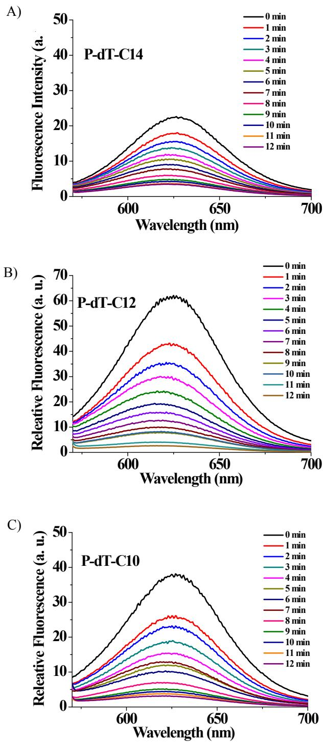
**Fig. S3** Fluorescence emission spectra ( $\lambda_{\text{exc}} = 550 \text{ nm}$ ) of the NR loaded aqueous solutions of A) P-dT-C<sub>14</sub>, B) P-dT-C<sub>12</sub> and C) P-dT-C<sub>10</sub> (10 mM) under UV irradiation (350-380 nm, 50 mW/cm<sup>2</sup>).
