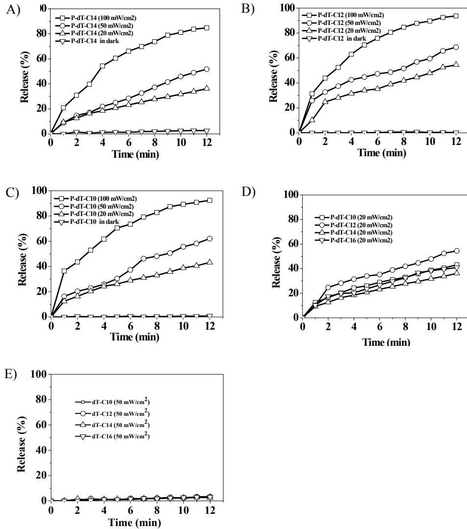
**Fig. S4** NR Release profiles of the NR loaded A) P-dT-C<sub>14</sub>, B) P-dT-C<sub>12</sub> and C) P-dT-C<sub>10</sub> solutions under UV irradiation at light intensities of 20, 50, and 100 mW/cm<sup>2</sup> and in the dark; D) Release profiles of NR in the P-dT-C<sub>n</sub> solutions under UV irradiation of 20 mW/cm<sup>2</sup>; E) Release profiles of NR in the dT-C<sub>n</sub> solutions under UV irradiation of 50 mW/cm<sup>2</sup>.
