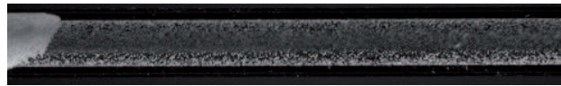
FIG. 9: Increase of the plug resistance to motion due to particles collection: Movie showing stick slip motion of the gas finger once it has reached a critical size. Time is accelerated by a factor of 15. This movie illustrates Fig. 9 of the manuscript.
