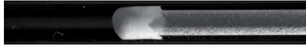
FIG. 8: Increase of the plug resistance to motion due to particles collection: Movie showing the slow down of a liquid plug pushed at constant flow rate \delta P = 0.2 kPa inside a capillary tube covered with particles (wetting conditions correspond to regime 2). This first movie shows the decrease of the plug velocity due to Coulomb friction of particles with the walls. Time is accelerated by a factor of 2. This movie illustrates Fig. 9 of the manuscript.
