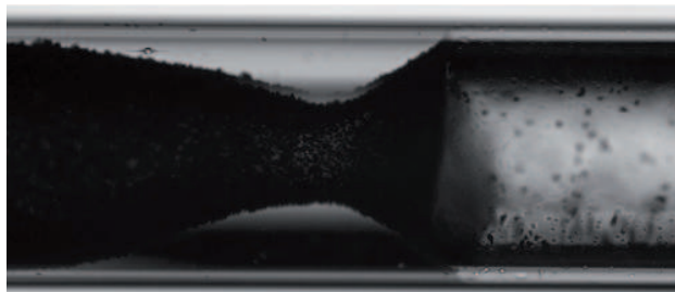
FIG. 5: Regime 2 : Movie in real time showing the pinch-off of the encapsulated gas finger. This movie illustrates Fig. 6 D of the manuscript.
