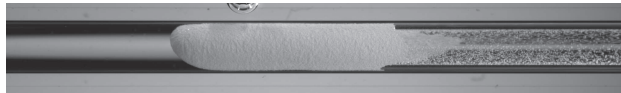
FIG. 4: Regime 2 : Movie showing the formation and growth of the gas finger encapsulated inside a monolayer of particles. Time is accelerated by a factor of 10. This movie illustrates Fig. 6 C of the manuscript.
