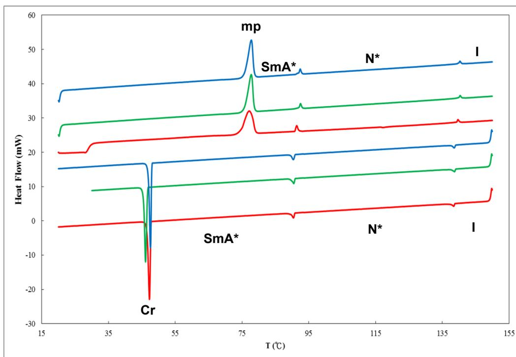
**Fig S3.** The DSC thermograms of 1<sup>st</sup> heating-cooling (red-traces), the 2<sup>nd</sup> heating-cooling (green-traces) and 3<sup>rd</sup> heating-cooling (blue-traces) cycles obtained from compound **HI** ( $n=7$ ).
