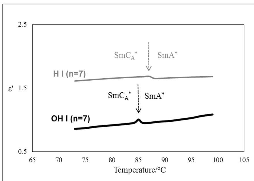
**Fig S6.** Temperature dependence of the dielectric constant  $\epsilon'$  for compounds **OH I** (n=7) and **H I** (n=7) at 100 Hz in the cell with 25 μm thickness under 1°C min<sup>-1</sup> cooling process.
