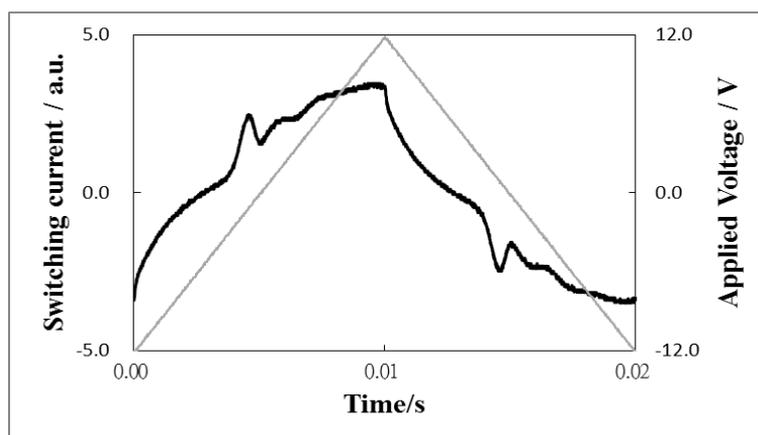
**Fig S4.** Switching current in a triangle electric field (50 Hz, 5 V<sub>pp</sub>) in the SmC<sub>A</sub>\* phase at 82.0 °C for compound **OH I** (n=7) in 5 μm thickness of homogeneously aligned cell.
