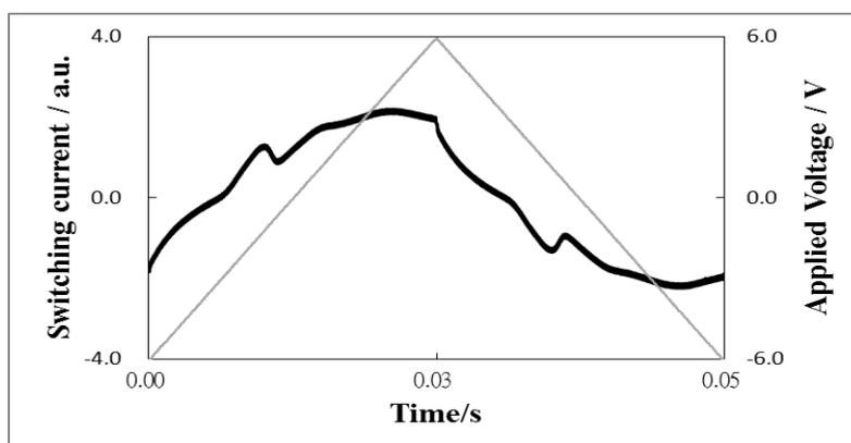
**Fig S5.** Switching current in a triangle electric field (20 Hz, 4 V<sub>pp</sub>) in the SmC<sub>A</sub>\* phase at 78.0 °C for compound **H I** (n=7) in 5 μm thickness of homogeneously aligned cell.
