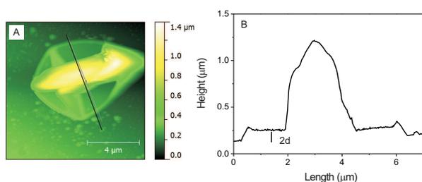
**Fig. S1** (A) AFM image of a dried shell, after removing the PDMS core by washing with ethanol. (B) The height profile taken along the line drawn through the collapsed capsules shows plateaus from which we obtained a shell thickness of  $d = 56$  nm.
