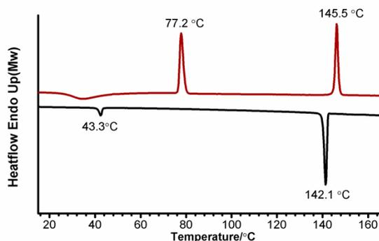
**ESI Fig. 1** DSC traces of compound **M3** on 2nd heating run (red line) and 1st cooling run (black line) at 10 °C/min under N<sup>2</sup>.
