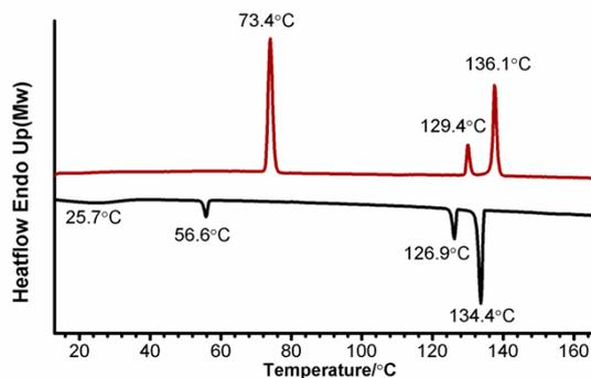
**ESI Fig. 3** DSC traces of compound **M5** on 2nd heating run (red line) and 1st cooling run (black line) at 10 °C/min under N<sup>2</sup>.
