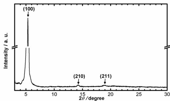
ESI Fig. 4 XRD pattern for  $Col_{hp}$  phase of **M5** on heating run at  $100^{\circ}C$
