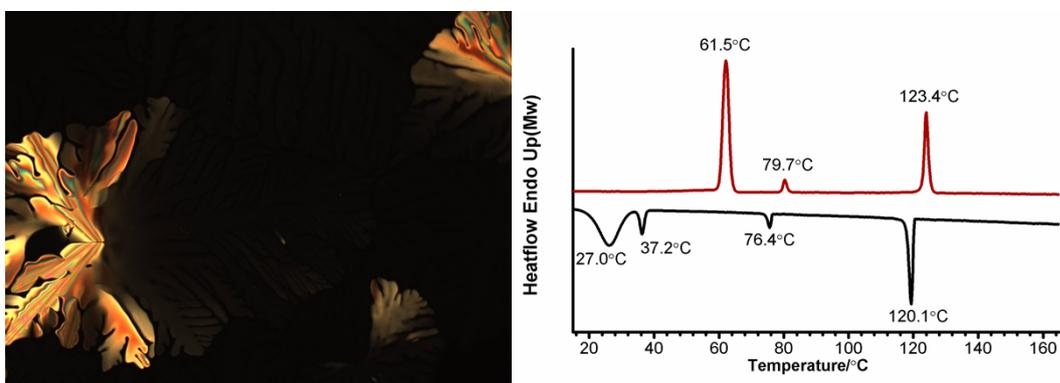
ESI Fig. 5 Dendritic texture of compound **M6** sandwiched between clean glass slides on cooling from isotropic phase at  $120^{\circ}C$  (left), this texture which indicated a  $Col_h$  phase was observed by POM with  $45^{\circ}$  angle and did not show any changes when cooled to crystal phase; DSC traces of compound **M6** on 2nd heating run (red line) and 1st cooling run (black line) at  $10^{\circ}C/min$  under  $N_2$  (right).
