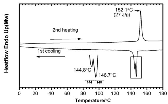
ESI Fig. 7 DSC traces of compound **D10** run at 10 °C/min under N<sup>2</sup>.
