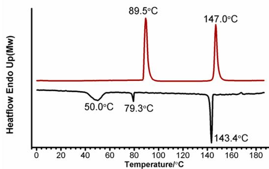
**ESI Fig. 2** DSC traces of compound **M4** on 2nd heating run (red line) and 1st cooling run (black line) at 10 °C/min under N<sup>2</sup>.
