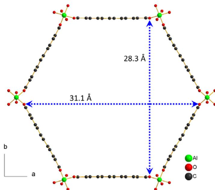
**Fig. S3.** The hexagonal pore sizes of CYCU-3.
