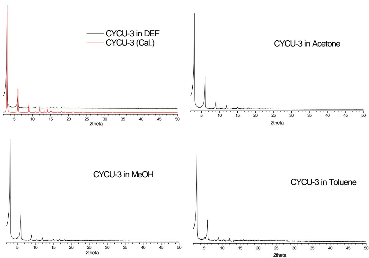
**Fig. S8.** Powder XRD patterns of **CYCU-3** treated with various solvents after desolvation.
