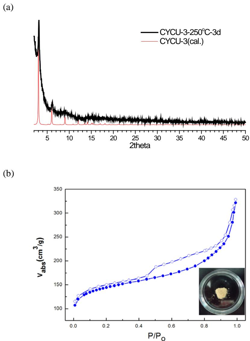
**Fig. S10.** (a) The powder XRD patterns for thermal treated samples of CYCU-3 by 250 °C and 3 days. (b) The N<sub>2</sub> sorption isotherms at 77K and photos of CYCU-3 after heated at 250°C and 3 days (solid circles, adsorption; open circles, desorption).
