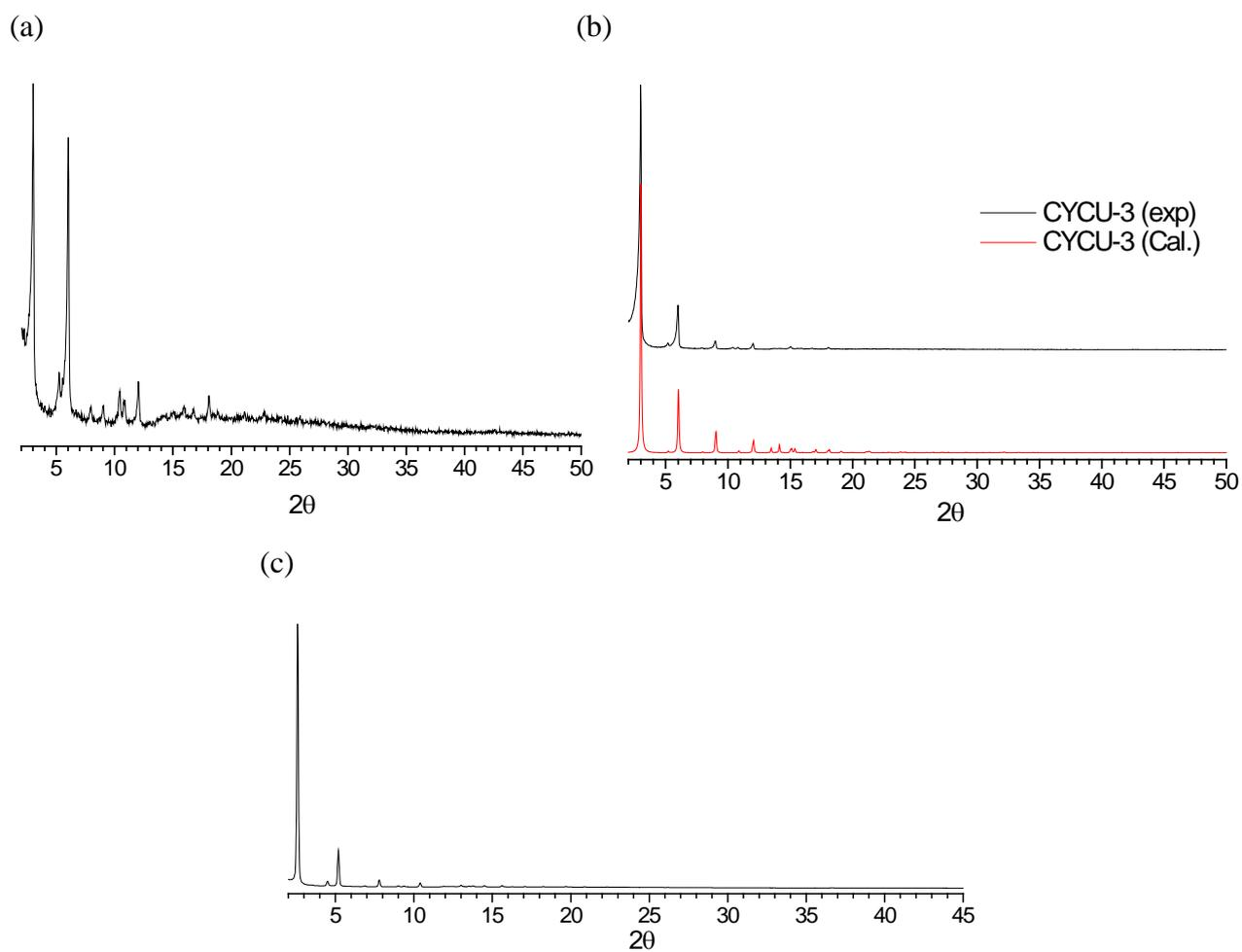
**Fig. S2.** Powder XRD patterns of: (a) as-synthesized CYCU-3; (b) desolvated CYCU-3; (c) desolvated CYCU-3 (measured by synchrotron radiation).
