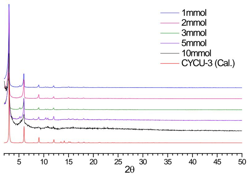
**Fig. S7.** Powder XRD patterns of **CYCU-3** synthesized under various molarity of acetic acid.
