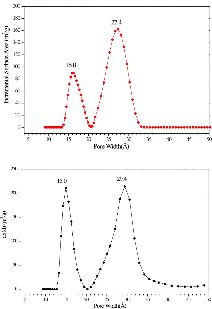
**Fig. S6.** The DFT pore size distribution of CYCU-3 analyzed from nitrogen sorption isotherms at 77K measured by the instruments of ASPA 2020 (top) and Autosorp-iQ (bottom).
