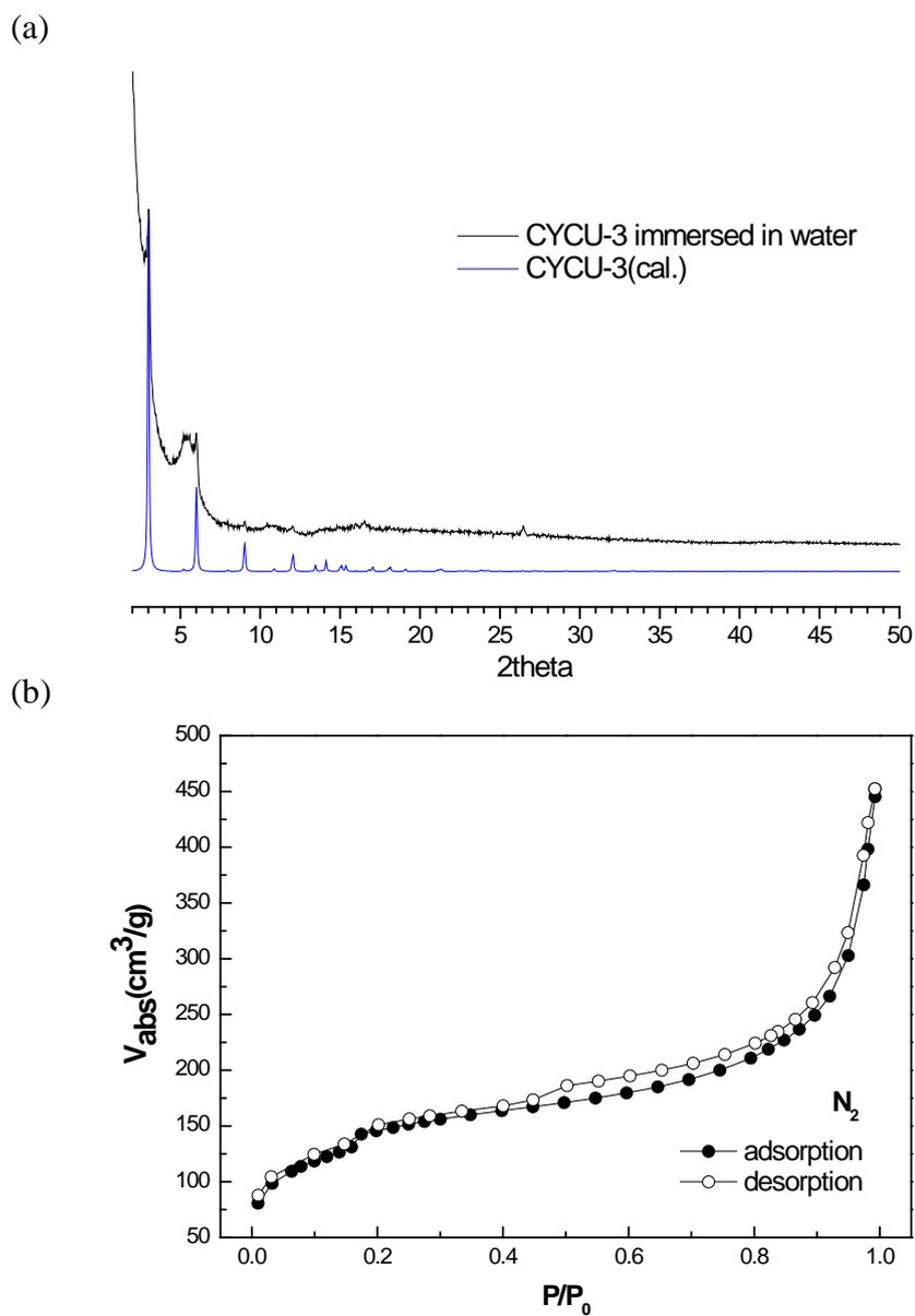
**Fig. S9.** (a) Powder XRD patterns of CYCU-3 sample after immerse in water for 7 day; (b) the nitrogen adsorption and desorption isotherms at 77 K of CYCU-3 after immersed in water and washed with water and hot DMF.
