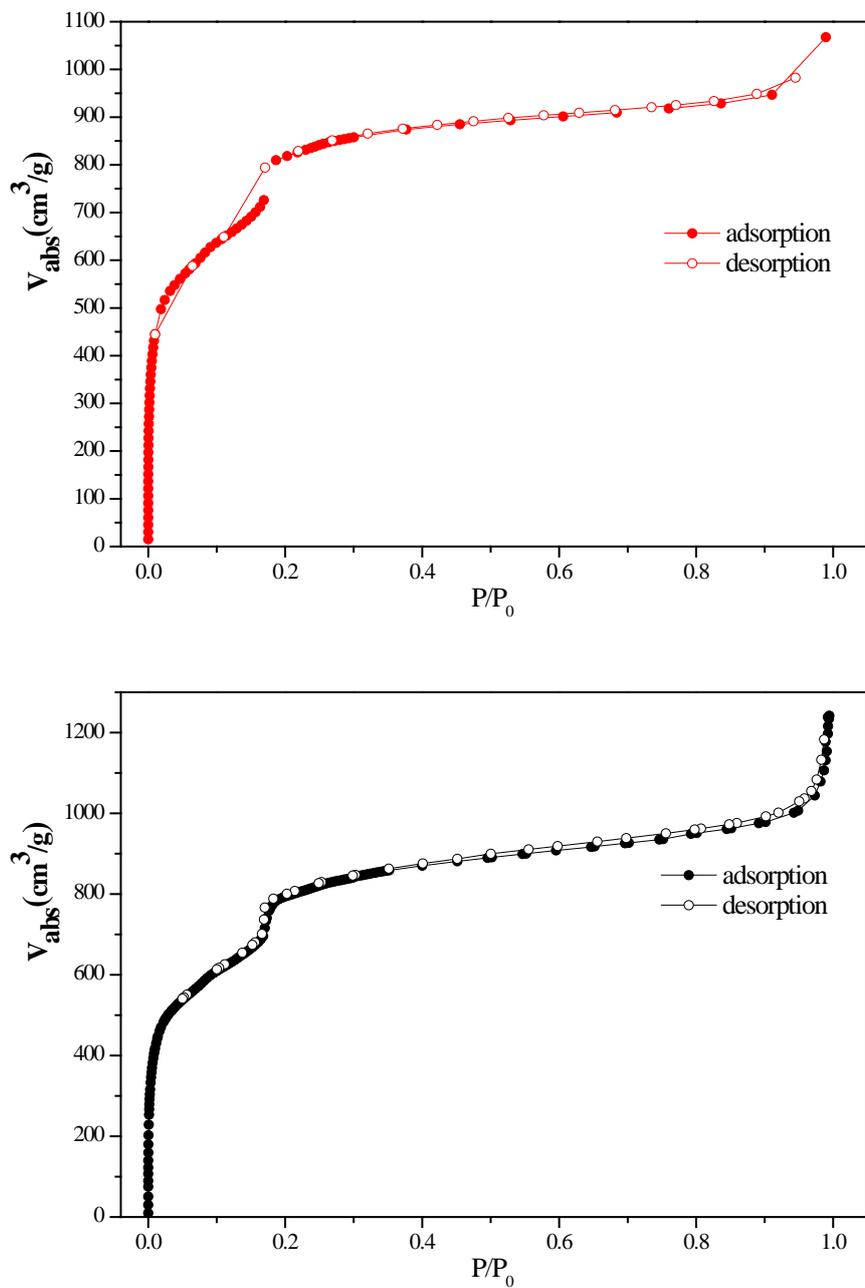
**Fig. S5.** Nitrogen sorption isotherms of CYCU-3 at 77K measured by ASAP 2020 (top) and Autosorp-iQ (bottom).
