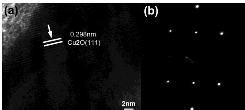
Figure S2. (a) HRTEM image and SAED pattern (b) of the shell of a hollow Cu<sub>2</sub>O nanocube.
