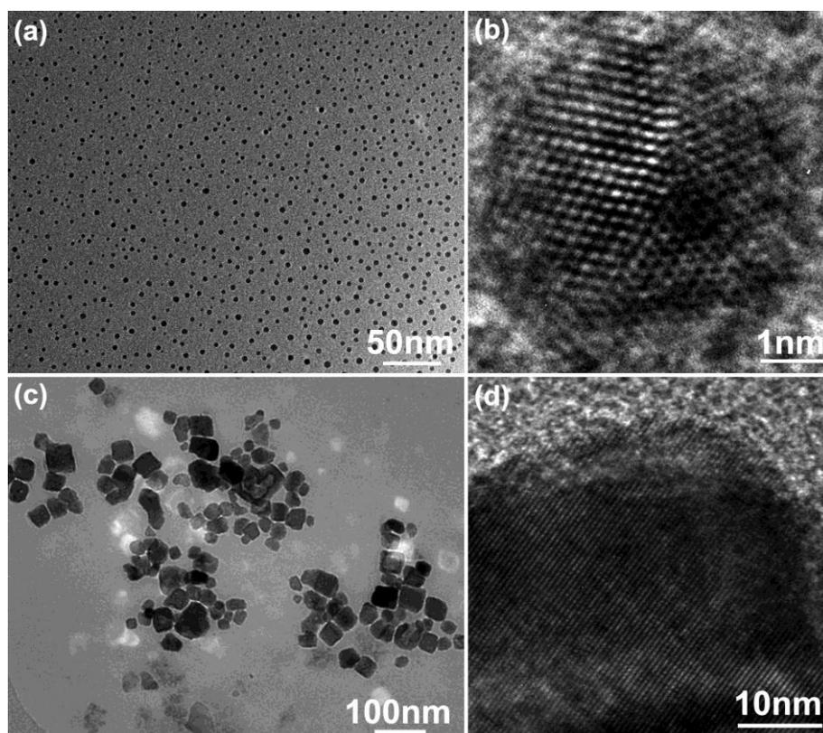
Figure S3. TEM images of the product of the reaction between CuCl and water at different pH values, (a) 4.3, (c) 8.5. HRTEM images of the product of the reaction of CuCl with water at different pH values, (b) 4.3, (d) 8.5.
