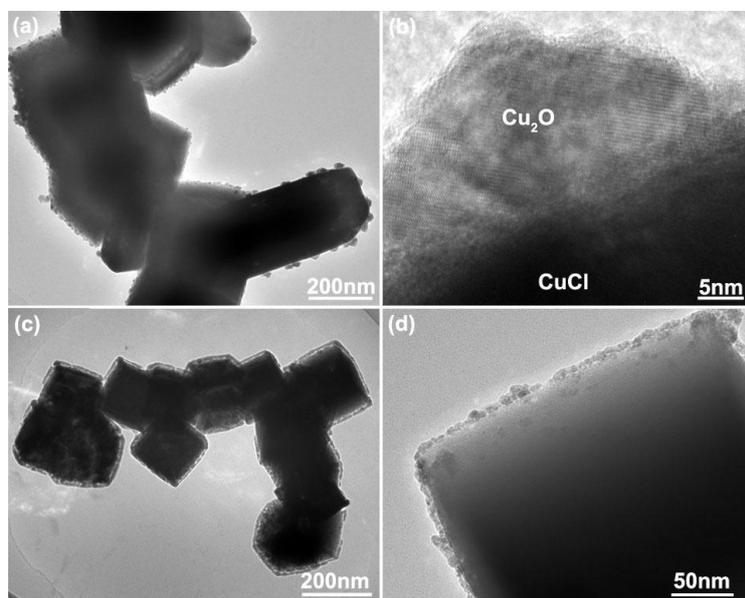
Figure S6 TEM images of the intermediate products obtained through the reaction of CuCl with water at pH of 6.5 for different times. (a) the product obtained after 2 min reaction, (b) high resolution TEM image of a Cu<sub>2</sub>O nanoparticle on a CuCl nanocube in (a), (c) the product obtained after 5 min reaction, (d) high magnification TEM image of a CuCl nanocube in (c).
