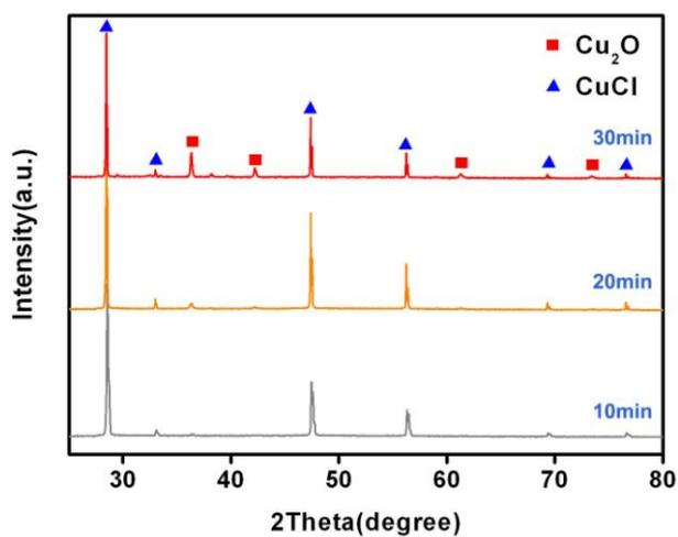
Figure S5. XRD patterns of the product after the reaction of CuCl with water (pH 6.5) for different times.
