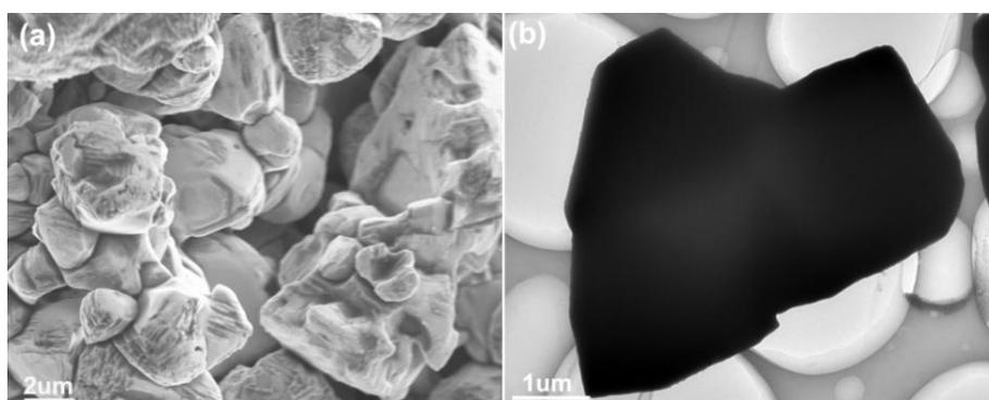
Figure S1. (a) SEM and (b) TEM images of raw CuCl micro-powder used as initial material.
