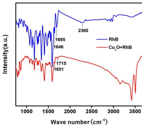
Figure S7. FTIR spectra of RhB and a mixture of hollow  $\text{Cu}_2\text{O}$  nanocubes and RhB.
