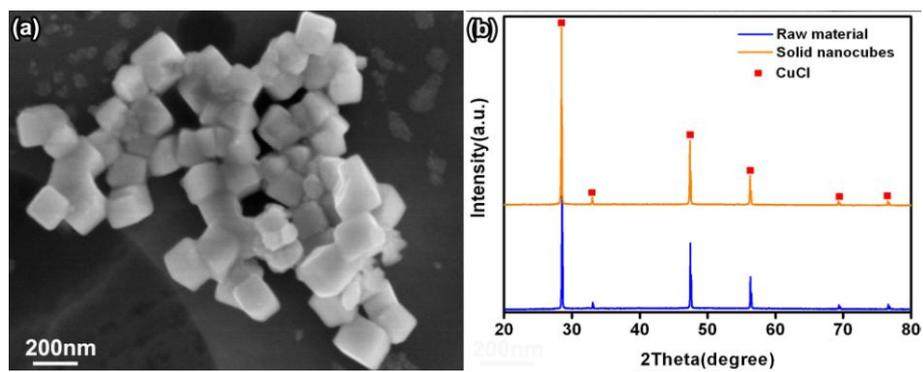
Figure S4. SEM image (a) and XRD pattern (b) of the CuCl nanocubes obtained after the dissolution of CuCl micro-powder in acidic water (pH= 0.5) followed by an increase in pH to 6.5 for a few seconds.
