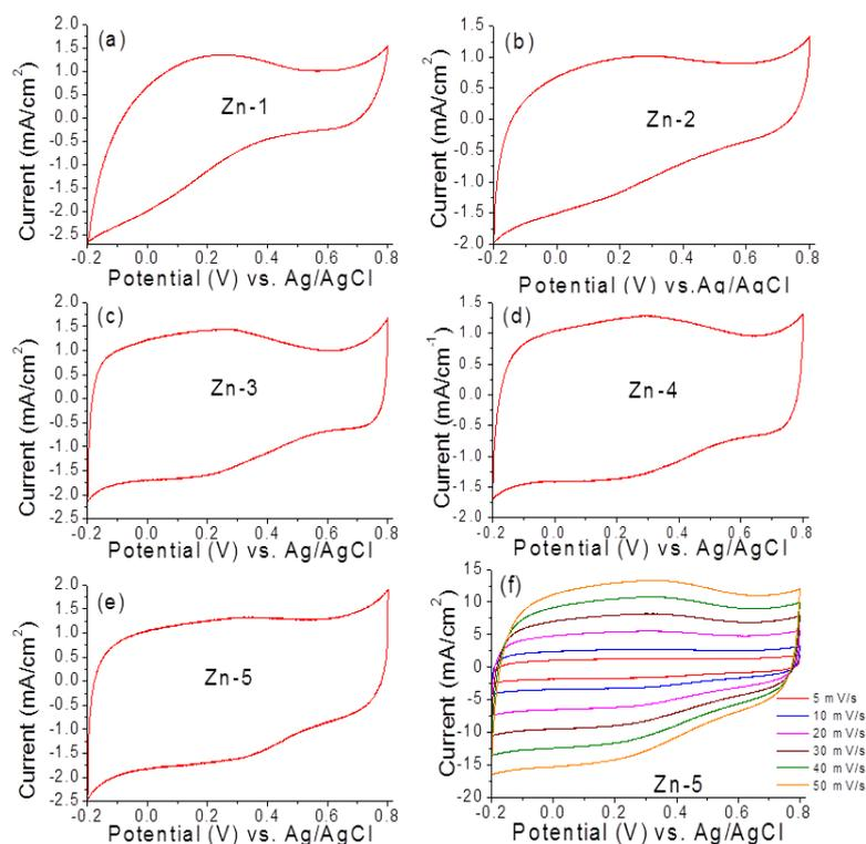
Fig. S3: CV curves of AC electrodes at 5 mV/s and Zn-5 at 5-50 mV/s.
