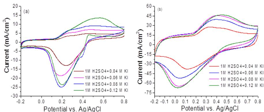
Fig. S4: CV curves optimized electrode (Zn-5) at (a) 5 and (b) 50 mV/s in different concentration of KI.
