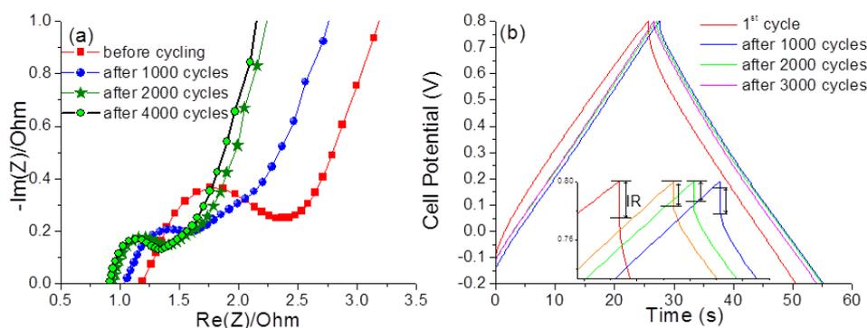
Fig. S8: (a) Nyquist plots and (b) charge discharge curves (at 5 mA cm<sup>-2</sup>) of AH at before and after cycles
