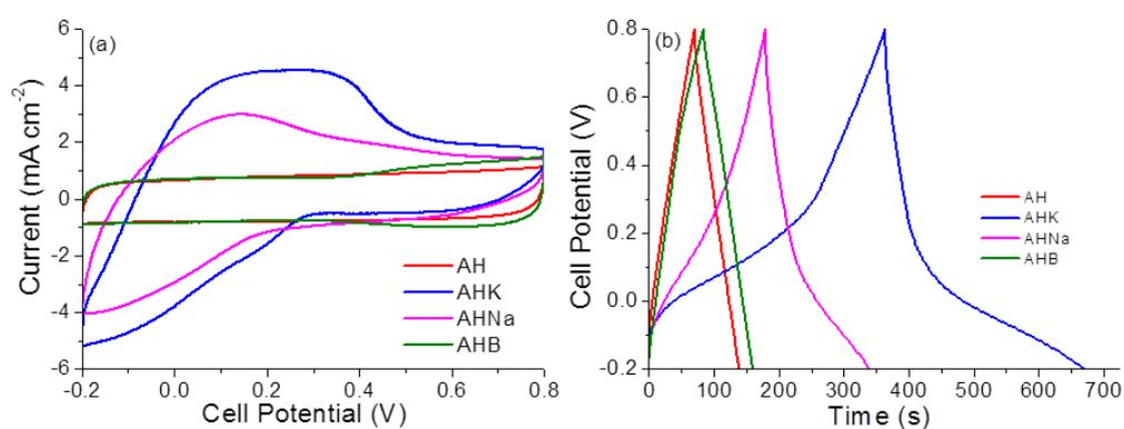
**Fig. S6:** CV curve and charge discharge curve of AH, AHK, AHNa and AHB at 5 mV/s and 2 mA cm<sup>-2</sup>.
