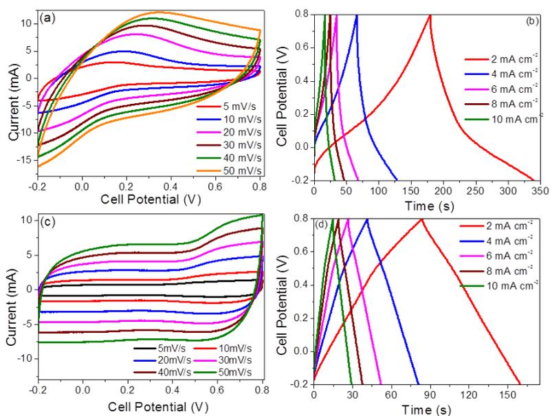
Fig. S7: (a, c) CV curves at 5-50 mV/s and (b, d) charge-discharge curves at 2, 4, 6, 8 and 10 mA cm<sup>-2</sup> of AHN and AHB
