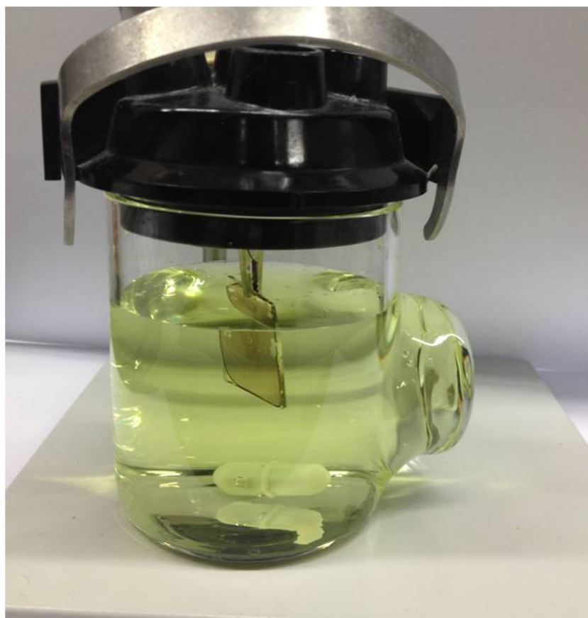
Fig. S4. Experimental setup for photocatalysis. C-ZnO film on Quartz substrate is suspended in PNP solution in quartz container. The experiment was conducted under stirring and the set up was exposed to light through the flattened window
