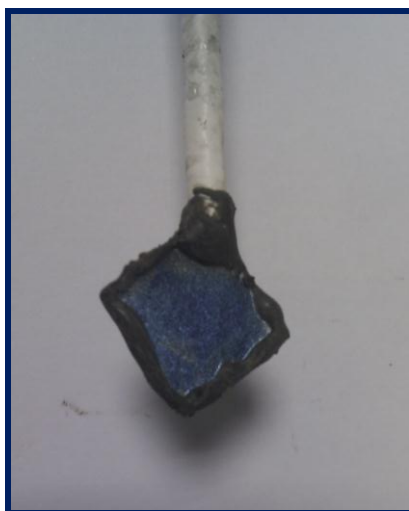
Figure S6. The vanadium foil obtained after drying in air. The foil was taken after electrochemical oxidation in NaCl aqueous solution for around 300 s.
