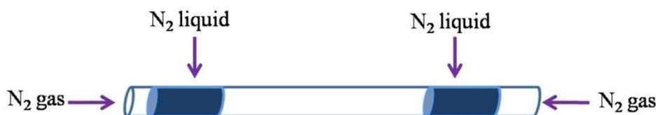
Scheme S1. A possible process of nitrogen liquefaction inside a long nanotube during BET measurement.
