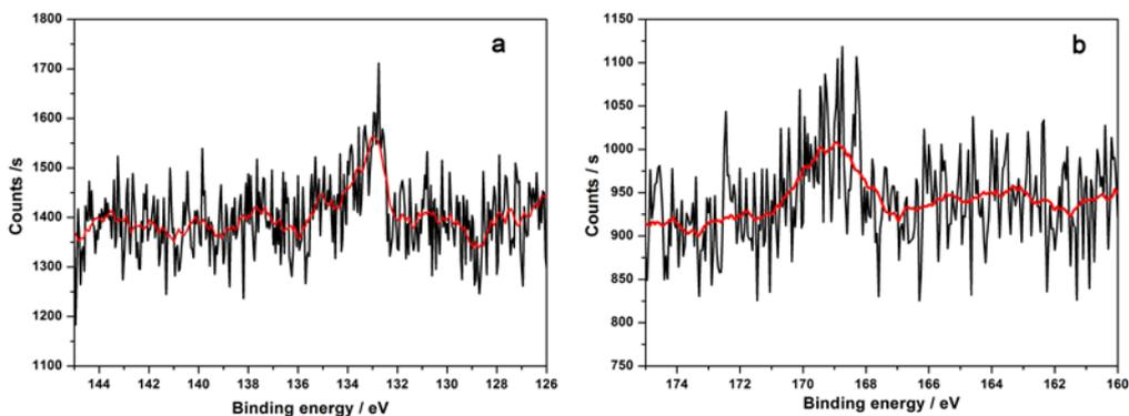
**Figure S1** The XPS spectrum of P atom in the P<sub>5</sub>W<sub>30</sub> based EC electrode (a) and the XPS spectrum of S atom in the S<sub>5</sub>W<sub>30</sub> based EC electrode (b).
