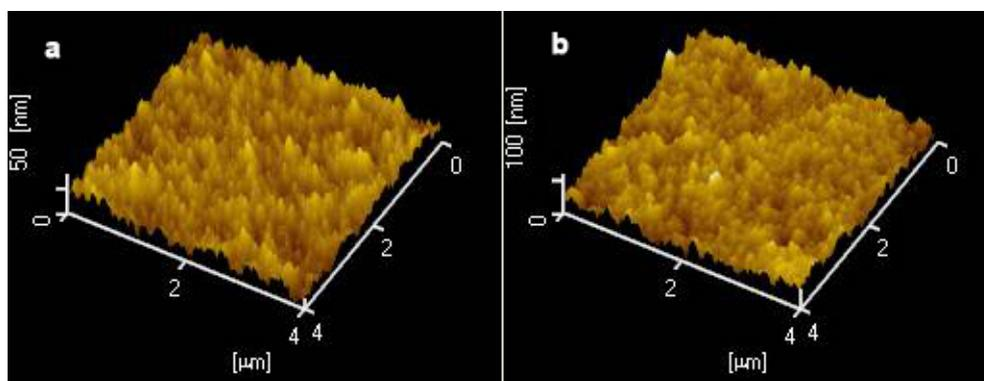
**Figure S7** the 3D AFM images of the P<sub>5</sub>W<sub>30</sub> (a) and S<sub>5</sub>W<sub>30</sub> (b) based EC electrodes.
