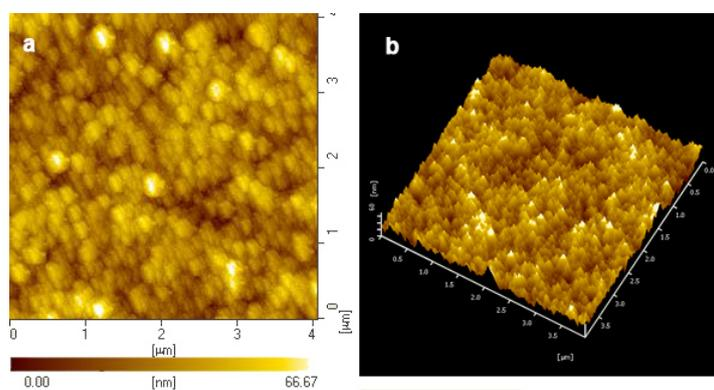
**Figure S6** the AFM image of the as-prepared TiO<sub>2</sub> film (a) and the the 3D AFM images of the as-prepared TiO<sub>2</sub> film (b).
