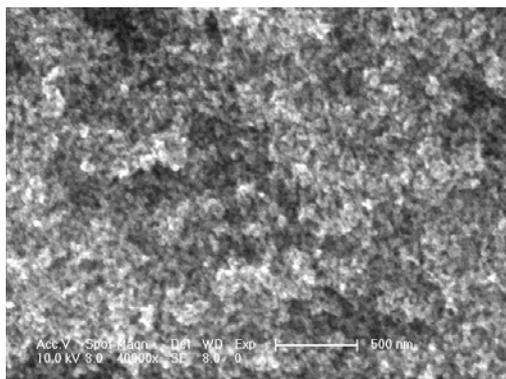
**Figure S5** the SEM image of the surface of the as-prepared TiO<sub>2</sub> film.
