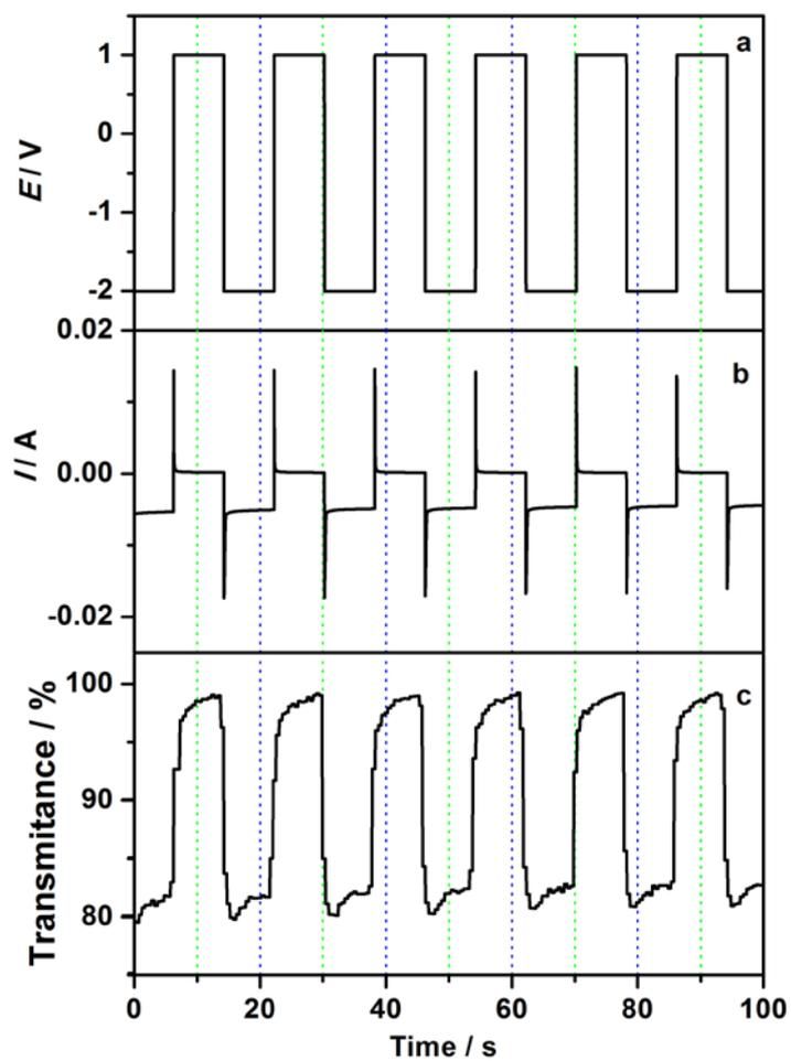
**Figure S9** Potential (a), current (b) and absorbance (c) at 550 nm of the smart window based on  $S_5W_{30}$  during the subsequent double-potential steps between 1.0 and -2.0V.
