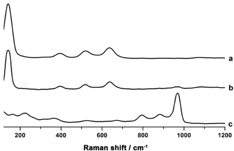
**Figure S3** Raman scattering spectra of bare TiO<sub>2</sub> substrate (a), P<sub>5</sub>W<sub>30</sub>-based electrode (b) and pure P<sub>5</sub>W<sub>30</sub> (c)
