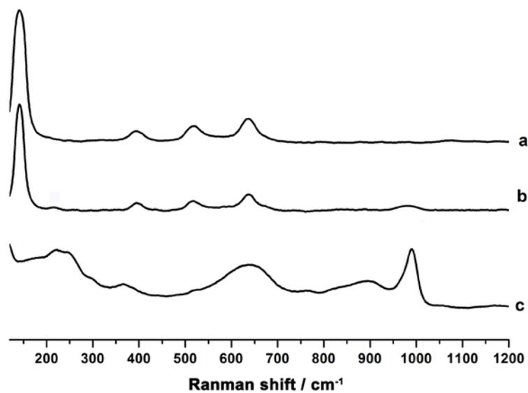
**Figure S4** Raman scattering spectra of bare TiO<sub>2</sub> substrate (a), S<sub>5</sub>W<sub>30</sub>-based electrode (b) and pure S<sub>5</sub>W<sub>30</sub> (c)
