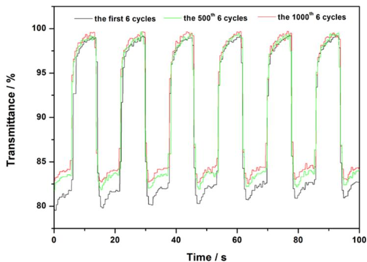
**Figure S10** The stability and reversibility of the  $S_5W_{30}$ -based smart windows. The black line represents the first 6 cycles of the double-potential steps; the green line represents the 500<sup>th</sup> 6 cycles of the double-potential steps; the red line represents the 1000<sup>th</sup> 6 cycles of the double-potential steps.
