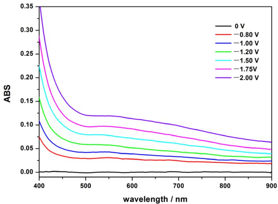
**Figure S8** Visible spectra of the smart window based on  $S_5W_{30}$  under different potentials ranging from -0.8 to -2.0V.
