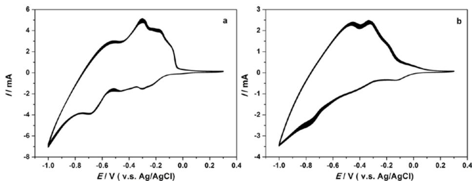
**Figure S2** The 100 cycles of CV test of the P<sub>5</sub>W<sub>30</sub>/TiO<sub>2</sub> (a) and S<sub>5</sub>W<sub>30</sub>/TiO<sub>2</sub> (b) film in LiClO<sub>4</sub> aqueous solution. (pH=3 adjusted by HCl)
